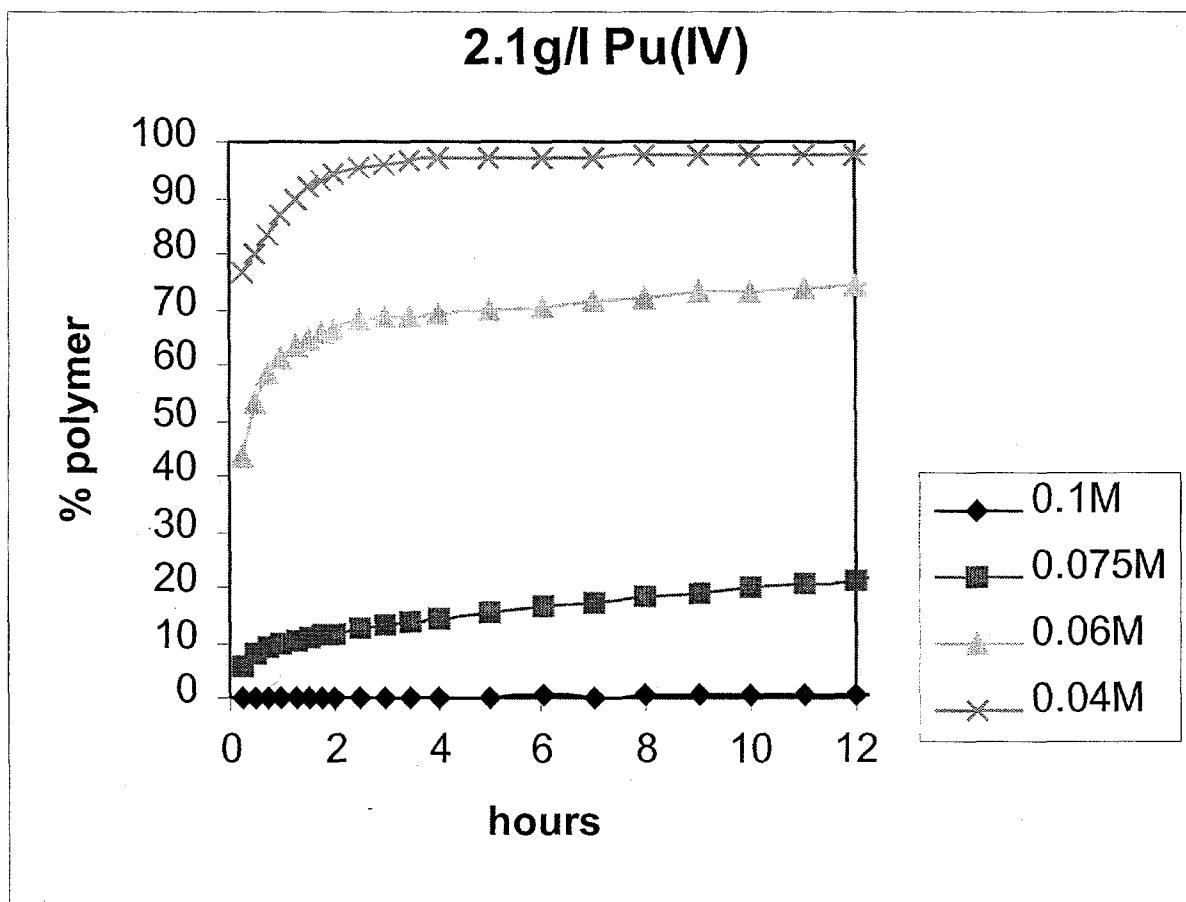
**Figure 3.** Rate of polymerization for 2.1g/L Pu in  $\text{HNO}_3$ .<sup>17</sup>
