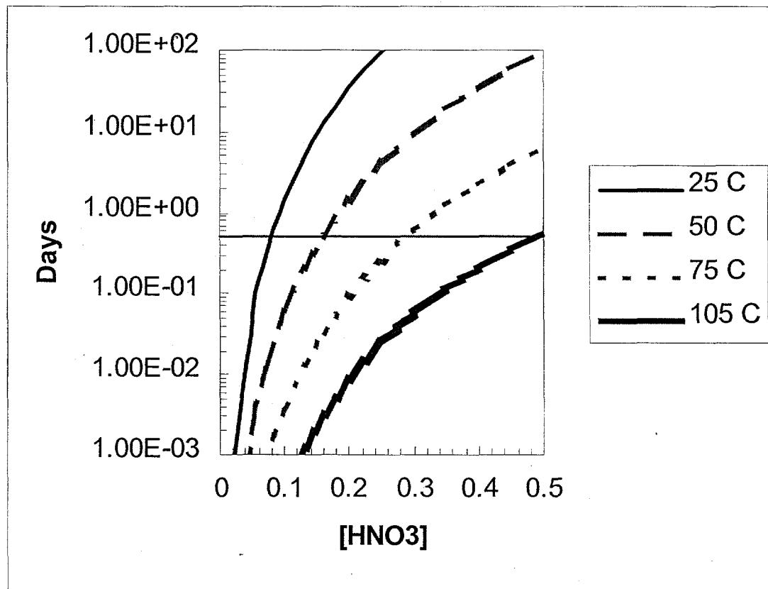
Figure 5. Rate of 2% polymer formation at 2g/L Pu as calculated from equation 7.<sup>25</sup>
