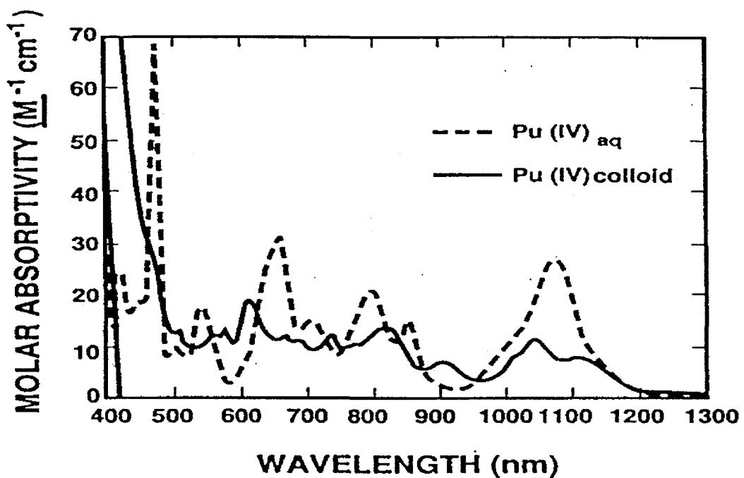
Figure 2. Absorption spectra of Pu(IV) and Pu(IV) polymer solutions.<sup>5</sup>
