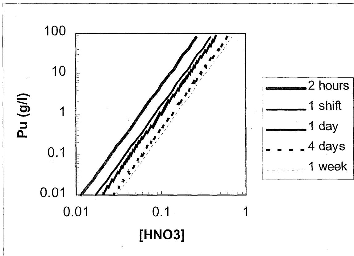
Figure 6. Rate of polymerization at 35°C as a function of Pu concentration as calculated from equation 7.<sup>25</sup>
