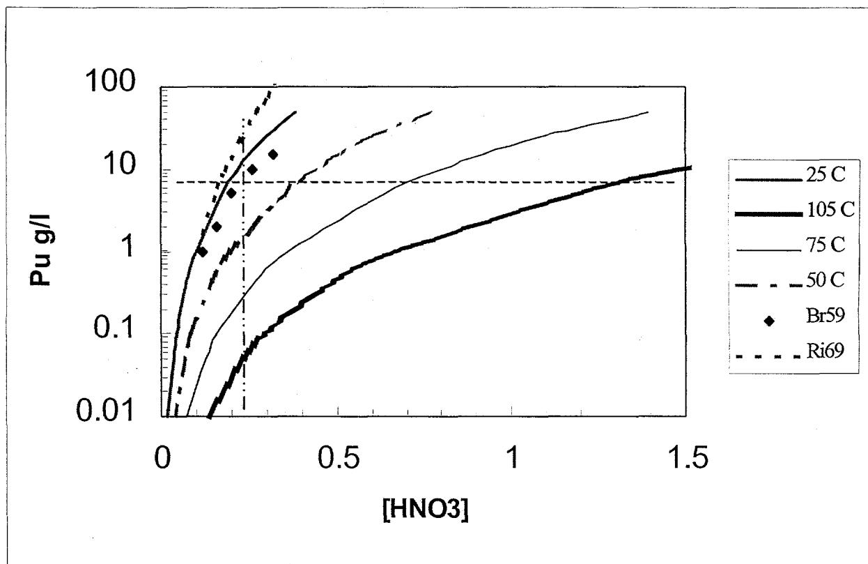
**Figure 4.** Effect of temperature on minimum  $\text{HNO}_3$  concentration required to prevent polymer formation calculated from empirical equations  $7^{25}$  and  $8^{26}$ . Equation 8 values, labeled Ri69, were calculated at  $25^\circ\text{C}$ . Experimental data labeled Br59 is from Brunstad.<sup>7</sup> The horizontal dashed line at 7 g/L Pu and the vertical dot dashed line at 0.22 M are process limits.
