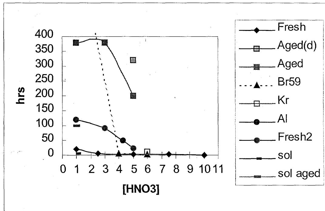
**Figure 7.** Depolymerizaton half times of fresh and aged Pu polymer at room temperature or 25°C. Fresh polymer values are labeled Fresh<sup>8</sup>, Br59<sup>7</sup>, Fresh2<sup>29</sup>, and sol.<sup>13</sup> Aged polymer values are labeled Aged(d)<sup>8</sup>, Aged<sup>29</sup>, Kr<sup>27</sup>, Al<sup>27</sup>, and sol aged.<sup>13</sup> Values labeled Aged were determined at 18°C.
