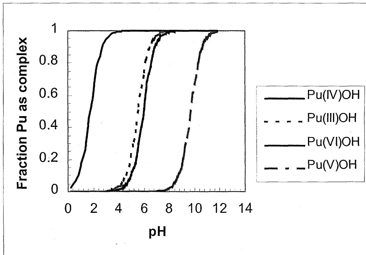
**Figure 1.** Onset of plutonium hydrolysis calculated as a fraction of the total Pu concentration using stability constants for monohydroxy Pu complexes.<sup>4</sup>
