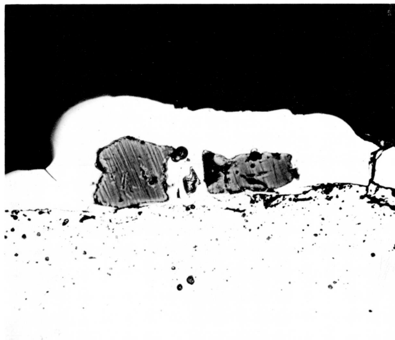
Figure 7 CATALYTIC PLATE SHOWING INCLUSIONS, HYDROGEN SULFIDE CATALYST, 500X MAGNIFICATION
