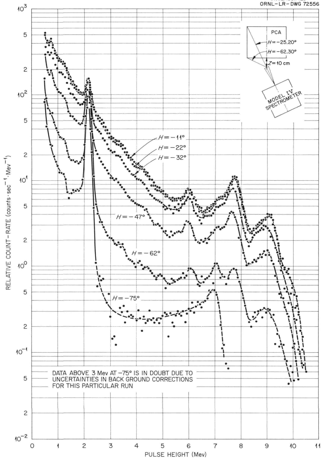
Fig. 1.1.6. Pulse-Height Distribution of Gamma Rays from a Stainless Steel Reactor Core at Various Angles About a Point in Water 10 cm from Core Surface.
