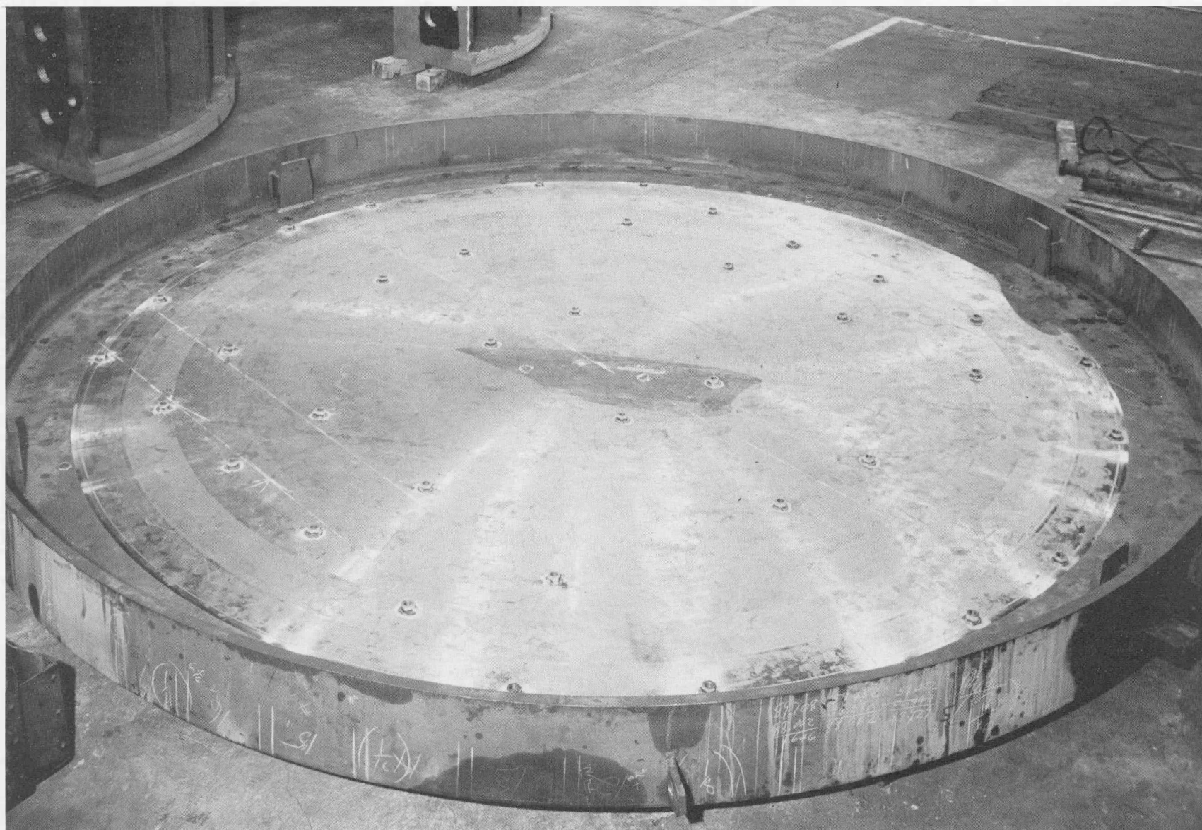
Figure 16. Containment Vessel Showing 2-in. Bottom Plate and Lower Shell Section. (ASTM - A-212 grade B steel)
