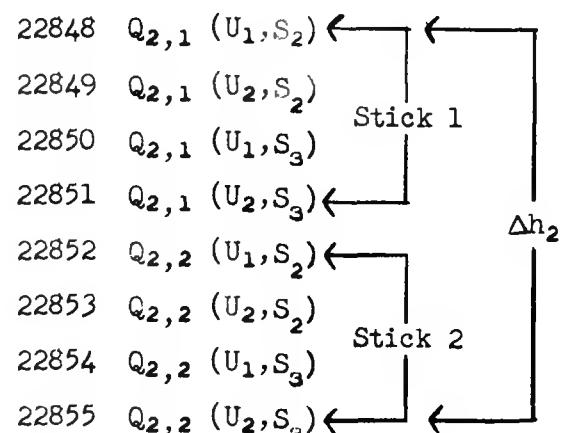
Primary Q input always starts at 18040 and ARD Q input starts at 22840. Q in the ARD input is always 4800 locations higher than its corresponding Q in the primary input. All Q input is in floating point form. The ARD input for height 1 could be omitted in this example because it is known that there will not be rods in an adjacent channel anywhere within this height. Thus, the first ARD input supplied would start at 22848.
