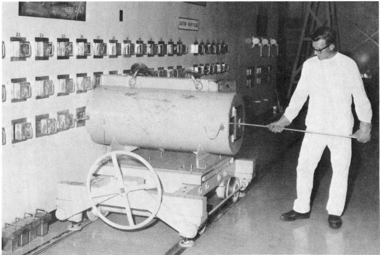
FIGURE 9: Standard Transfer Flask positioned in front of Horizontal Storage
