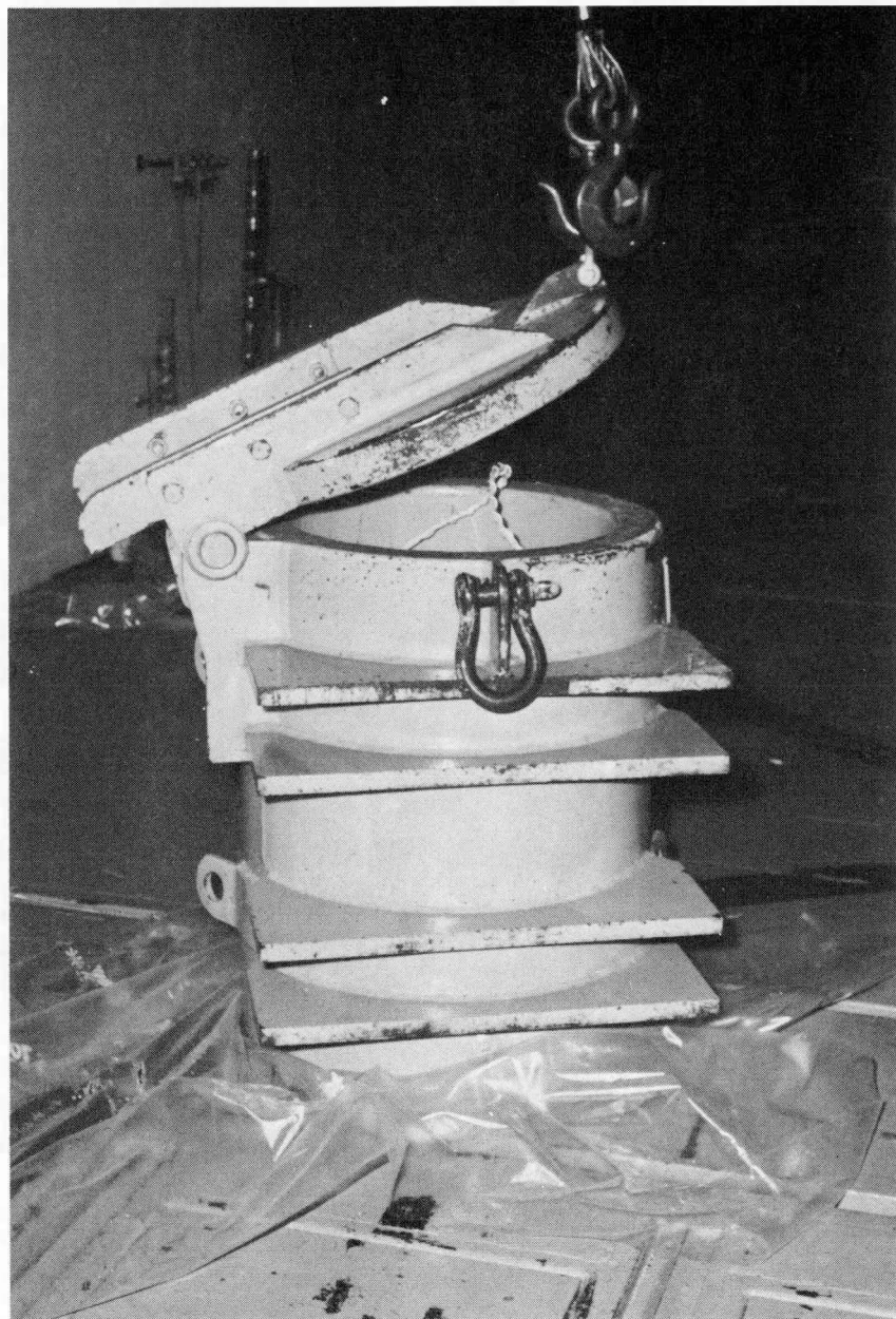
FIGURE 14: Garbage Can Flask with Lid in Partially Closed Position
