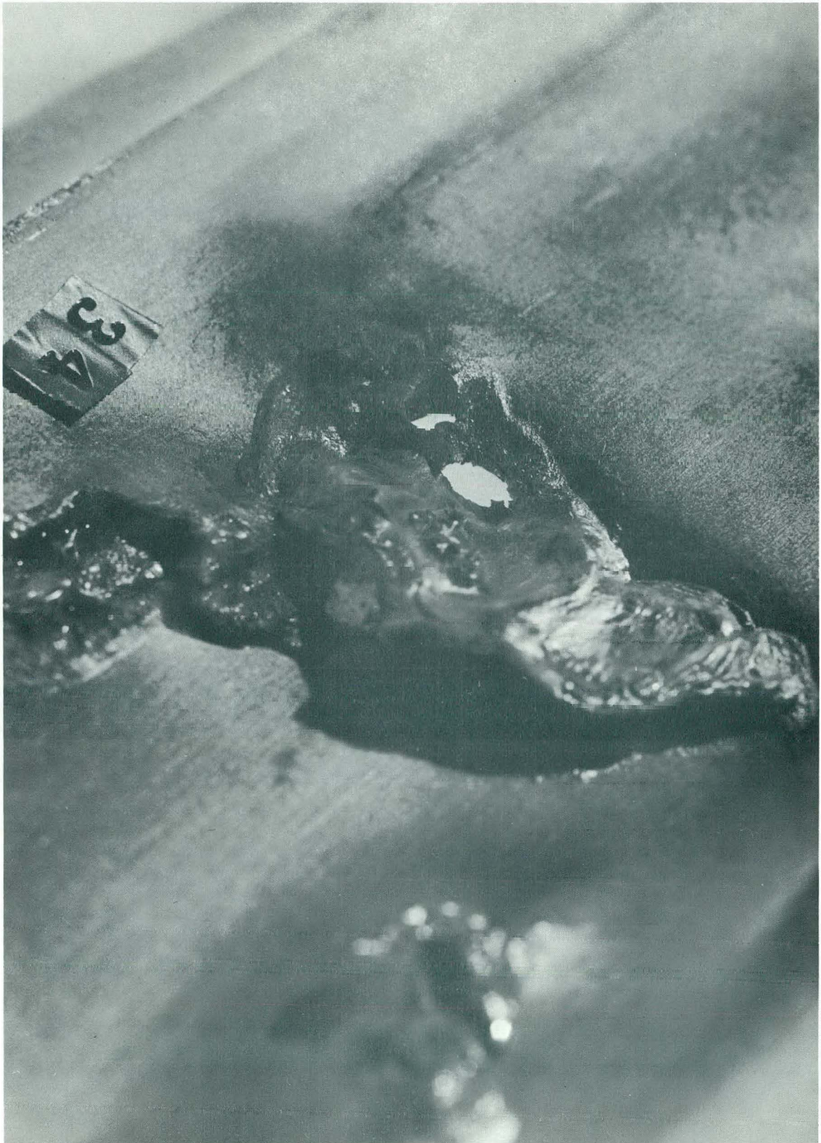
Fig. 28 Close-up view of melt showing hole through fuel plate (5-msec-period test).
