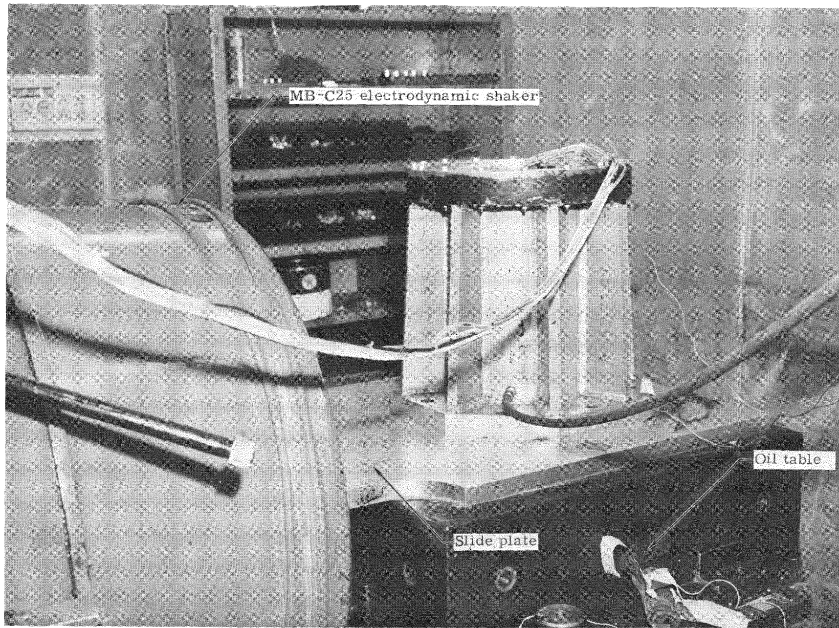
Fig. 34. Generator and Fixture Mounted to Slide Plate of Electrodynamic Shaker for Excitation in Horizontal Plane
