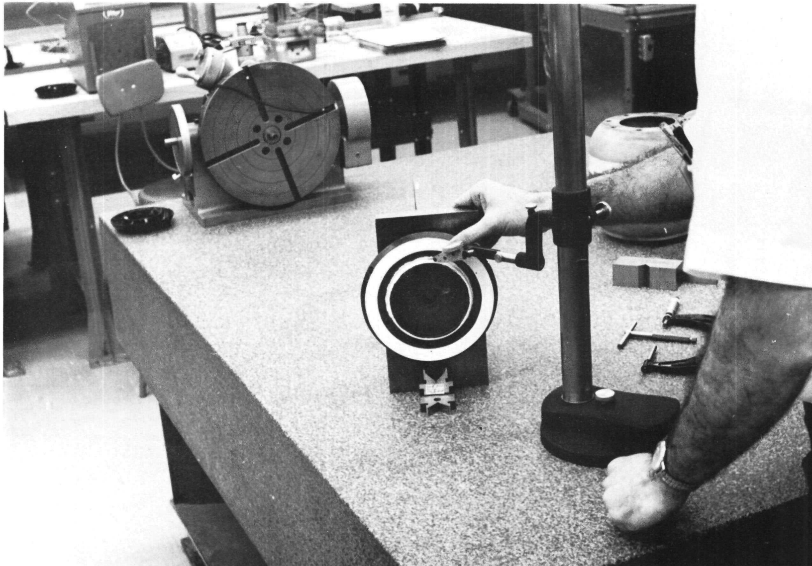
Figure 2-18. Inspection of the Spider, as Plasma Spray with Aluminum Oxide, Prior to Grinding for Interface with the Biological Shield
