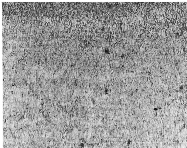
Figure S-89. 0.125 Thick — Hydroformed #8 — Top Sol'n Annealed at 2050°F for 10 Min ASTM Grain Size 4-1/2-6
