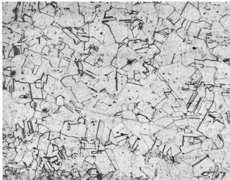
Figure S-99. 0.090 Thick - Hydroformed #7 - Top Sol'n Annealed at 2150°F for 10 Min ASTM Grain Size 4-5
