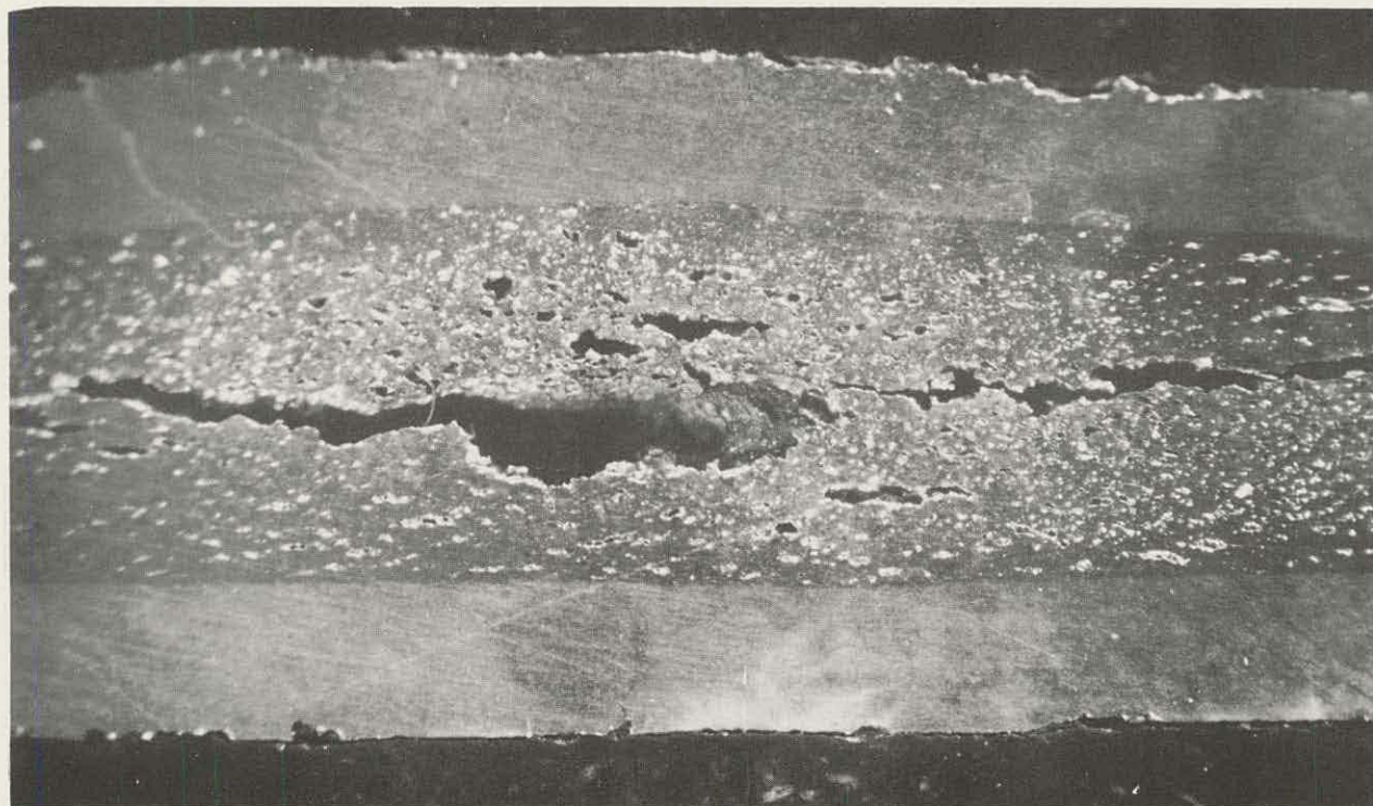
FIGURE 8. SECTION THROUGH SWELLED AREA OF ANL-2-11 Al-17.5 w/o U ALLOY FUEL PLATE
