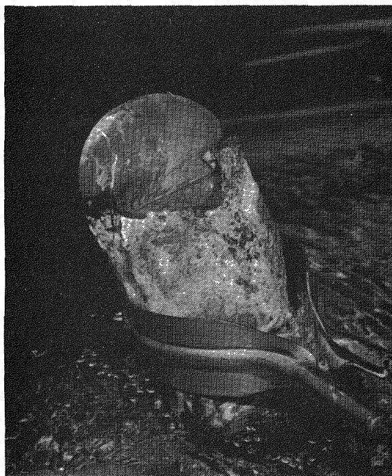
PHOTOGRAPH 29 - Exposed canistered capsule showing area that was broken to initiate canister sleeve removal.
