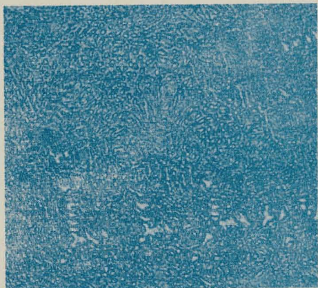
Fig. 3. - 9 wt % Mo-Th. Gamma molybdenum solid solution dendrites in a eu- tectic matrix. X750. Etchant: Murakamis' reagent.
