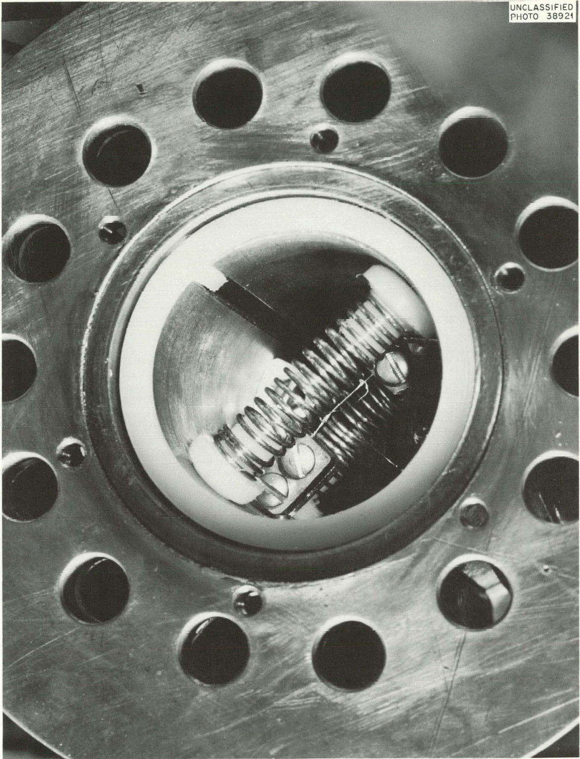
Fig. 7.12. Inside View of Test Cell for Resistance Measurements.
