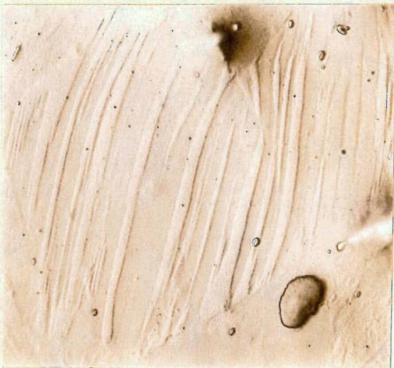
material. Accordingly, the effect of testing temperature on frequency of twinning was determined for a series of electro-refined specimens that had been deformed at the various testing temperatures at a head speed of 0.02 in./min. By using a point counting technique the results shown in Table II were obtained. From the table, it may be seen that the testing temperature has little effect on the frequency of twinning in the electrorefined plutonium, over the temperature range investigated.
