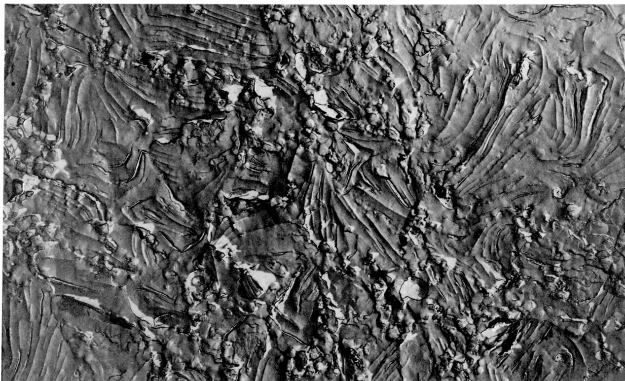
Fig. 5. Typical microstructure of extruded, resin-bonded graphite made from Santa Maria graphite flour, Lot ABS2. Xenon-ion etch, 5000X.
