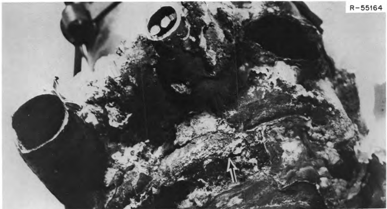
Fig. 13.31. Closeup of the bottom of freeze valve 105 showing the two gas outlet lines and one inlet line of type 304 stainless steel that was corroded completely. The crusty substance is the salt. Note that there is no salt in the air annulus.
