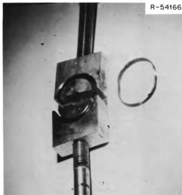
Fig. 13.11. Fixture used for pulling Hastelloy N rings cut from the control rod thimble.
