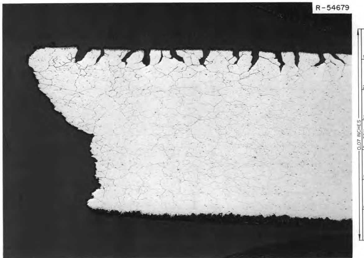
Fig. 13.12. Hastelloy N ring from control rod thimble stressed at 25°C. The cracked surface was exposed to the fuel salt, and the oxidized surface was exposed to the cell environment of 2 to 5% O 2 and N 2 .
