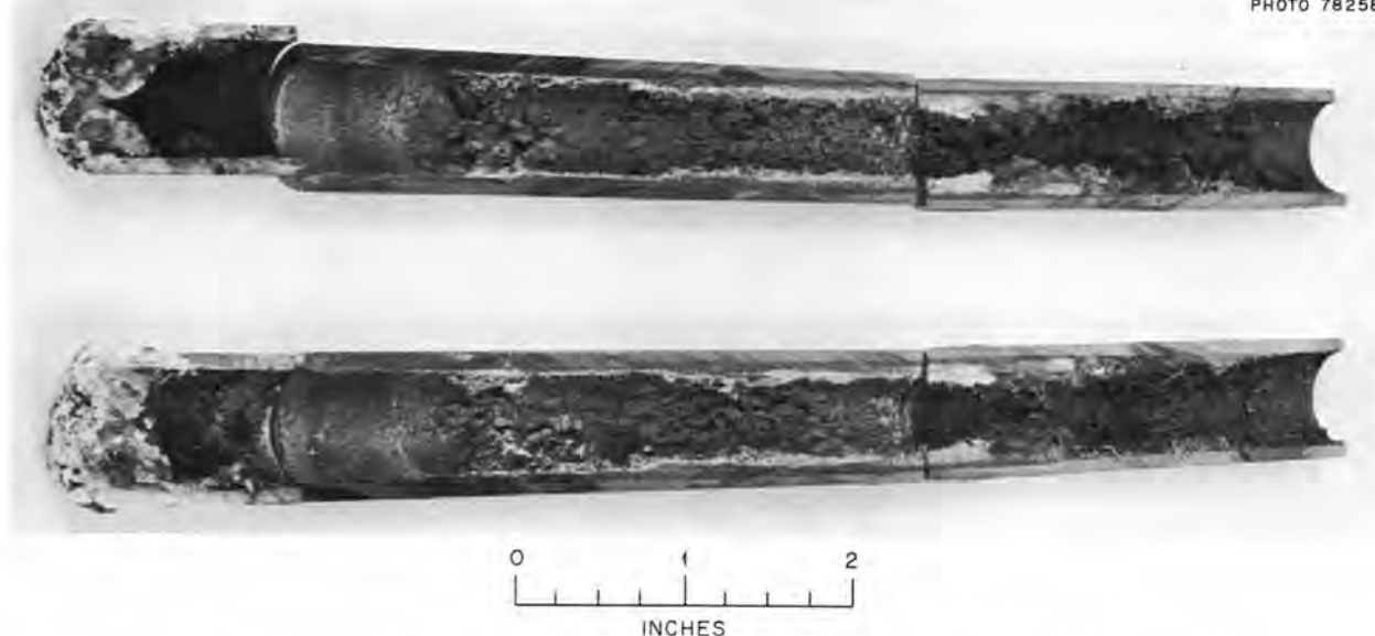
Fig. 5.7. Interior view of \text{BF}_3 feed and salt level bubbler tube, \text{NaBF}_4 circulation test, PKP loop, 9201-3.
