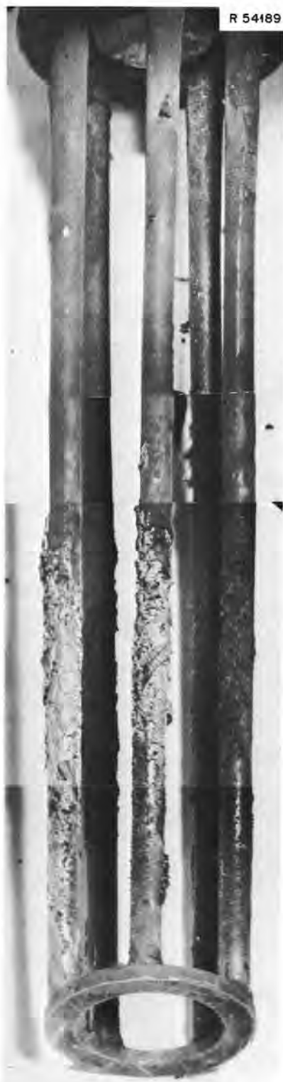
Fig. 8.5. Deposits on sampler cage. Ring already scraped.
