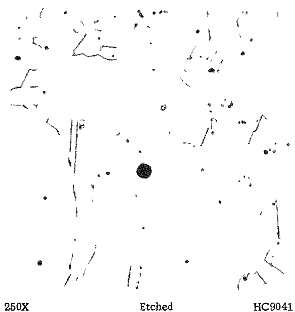
c. Center of Specimen LB-3-H Irradiated at 120 F to 6.5 \times 10^{21} NVT
