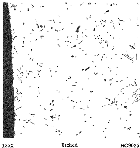
b. Inside Edge of Specimen LB-3-I Irradiated at 120 F to 4.5 \times 10^{21} NVT
