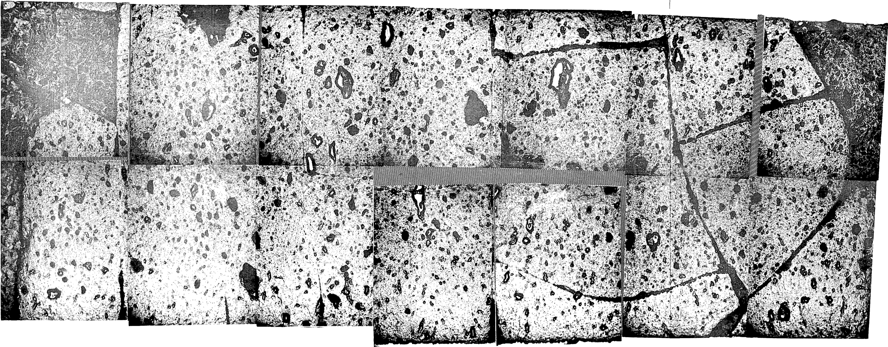
FIGURE 12. LONGITUDINAL SECTION THROUGH 70 WT % \text{UO}_2\text{-BeO} FUEL SPECIMEN
