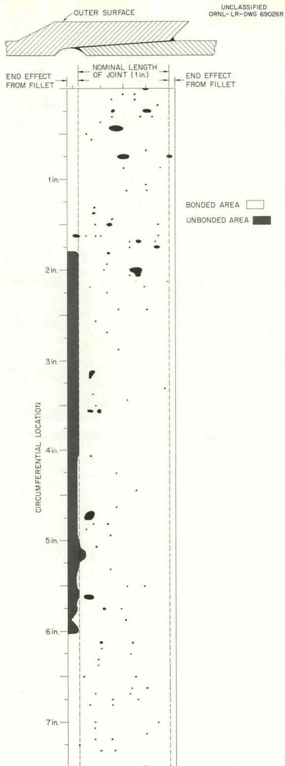
Fig. 4.6. Results of Ultrasonic Inspection of a Remotely Brazed Pipe Joint.
