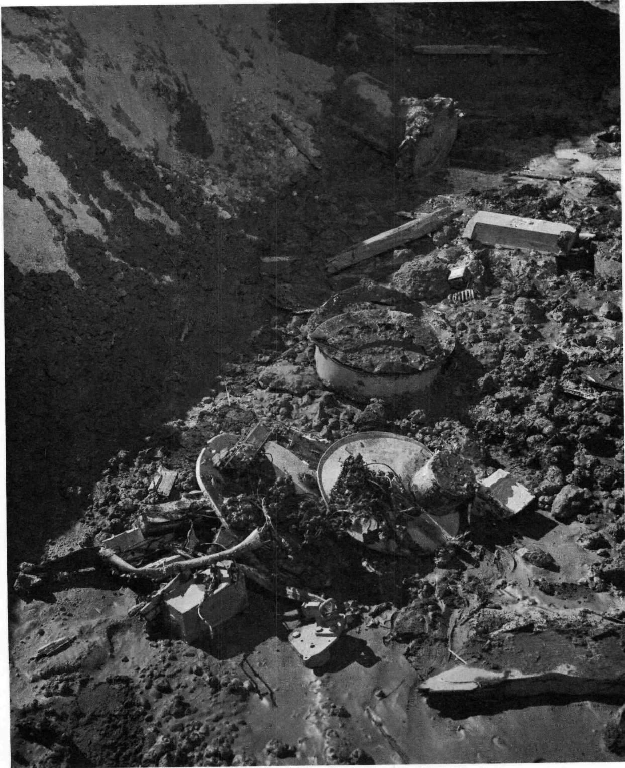
Figure 20. Debris Recovered After Head-On Water Impact
