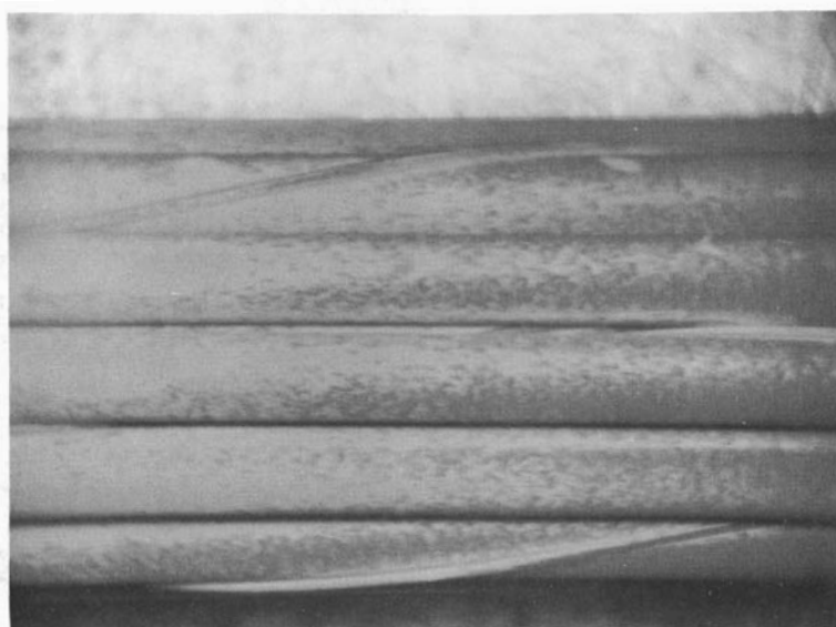
FIGURE 3.16. Fuel Rod Region of PRTR FE-5224 Showing Uniform Crud Deposition and the Crevice Corrosion on the Rod Surfaces Associated with the Circumferential Strip Bands that Occurred During Operation with LiOH-Controlled pH-9 Coolant
