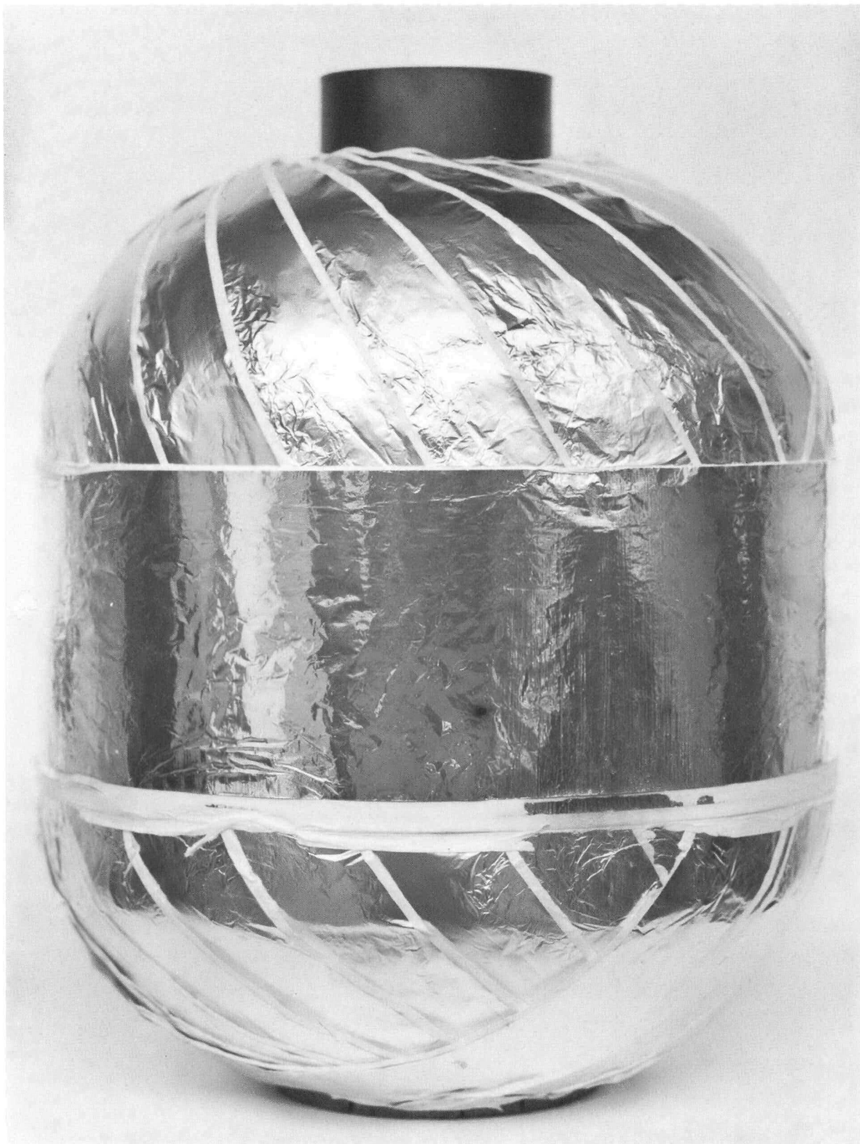
Figure 3-2. Wood Dummy of 10-Watt Configuration with Machine Applied Insulation (Neck Tube at Bottom of Photograph)
