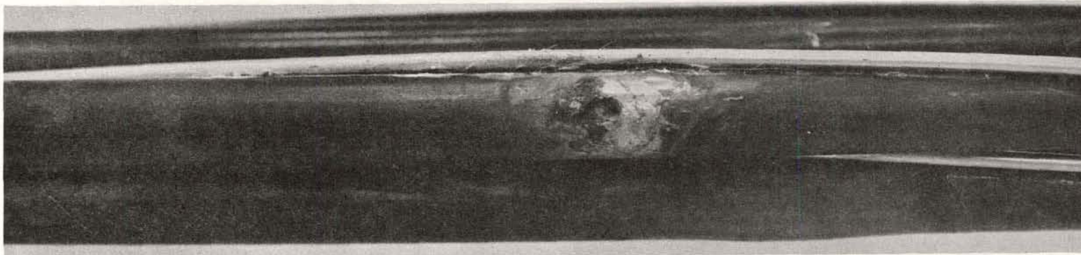
Figure 18. Melting of Cladding, Due to Burnout
