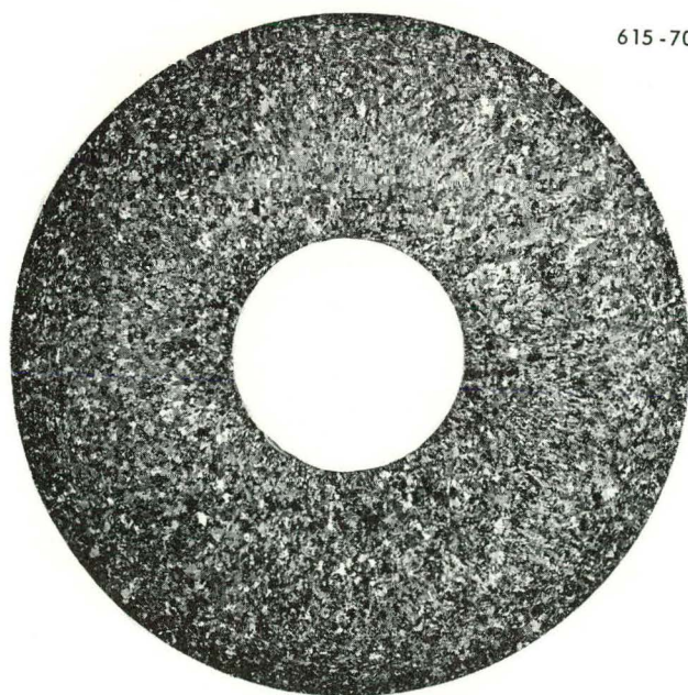
A – Billet No. P85, Transverse Section (1X)
