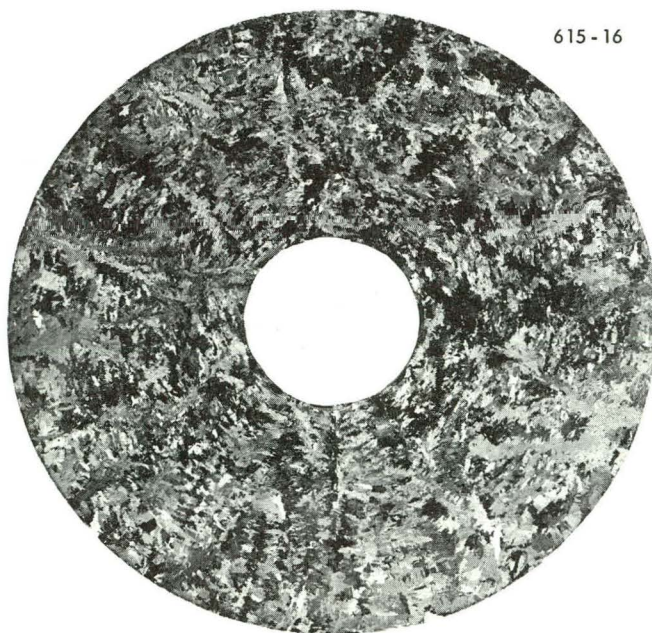
A – Billet No. P85, Transverse Section (1X)
