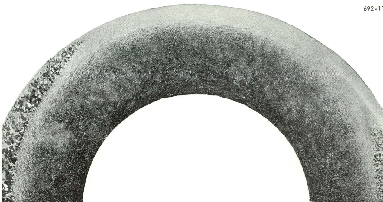
A – Small Alpha Grains on Portion of Outside Diameter; Billet No. 33284 B4 (Rear), Tube No. 33; Transverse Section (3X)
