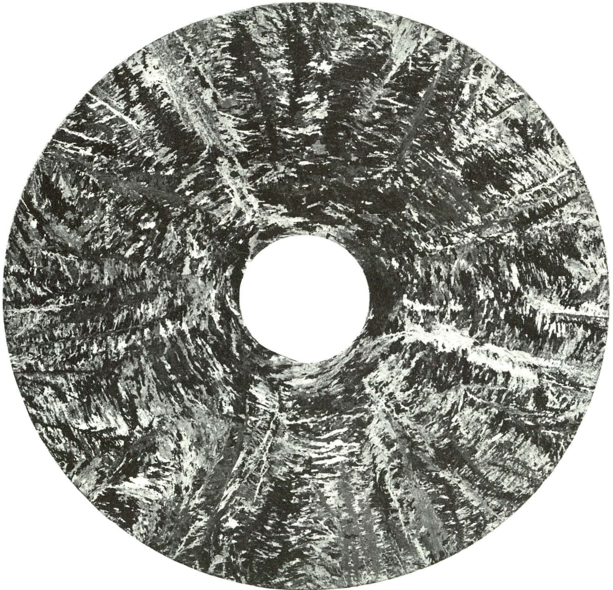
FIGURE 8 Typical, As-Cast, Alpha-Phase Grain Structure in Extrusion Billet ( 8\frac{3}{4} -inches OD by 1\frac{1}{4} -inches ID by 18-inches Long), Ingot No. 33277, Transverse Section. (0.7X)
