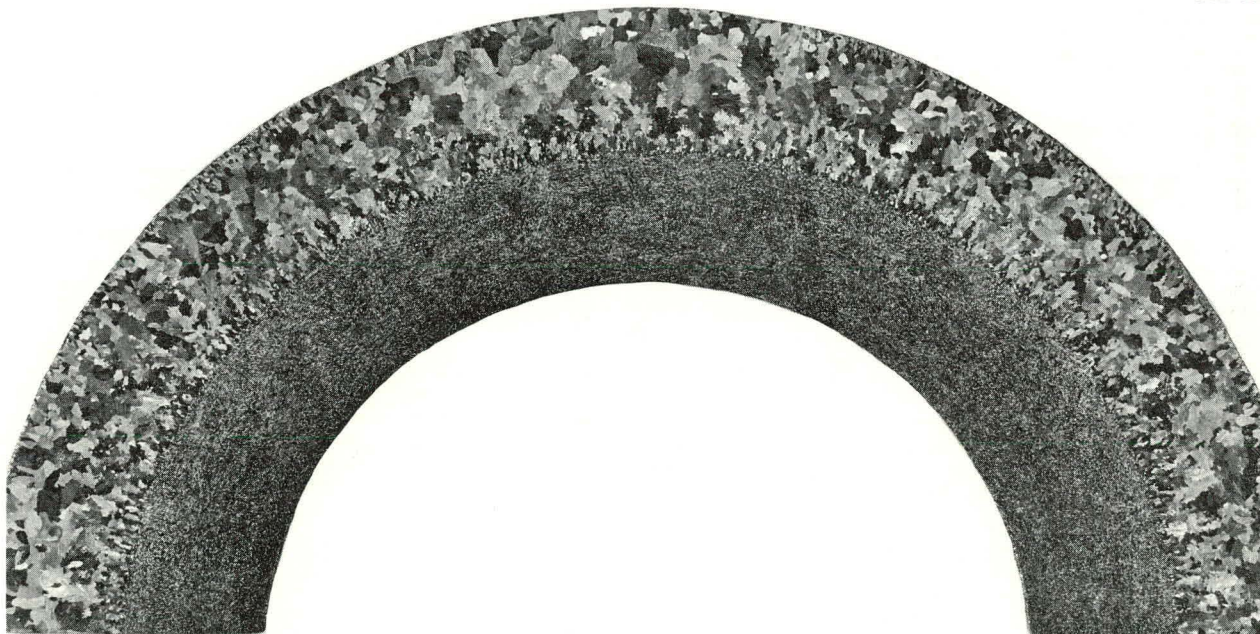
FIGURE 13 Duplexed Grain Structure in Statically Cast, Beta Heat-Treated, Extruded, and Rotary Elongated Tube; Medium-Size Alpha Grains on Outside Diameter; Billet No. 33298 T5 (Front), Tube No. 3, Transverse Section (3X)
