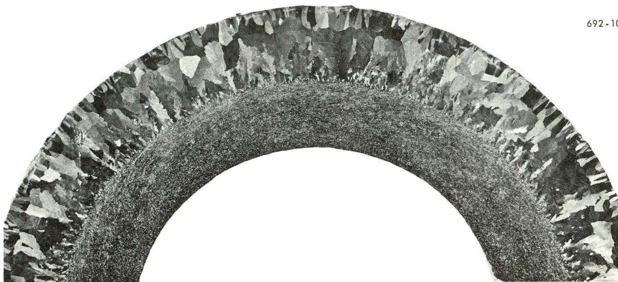
A – Coarse Alpha Grains on Outside Diameter; Billet No. 33284 T2 (Rear), Tube No. 25; Transverse Section (3X)
