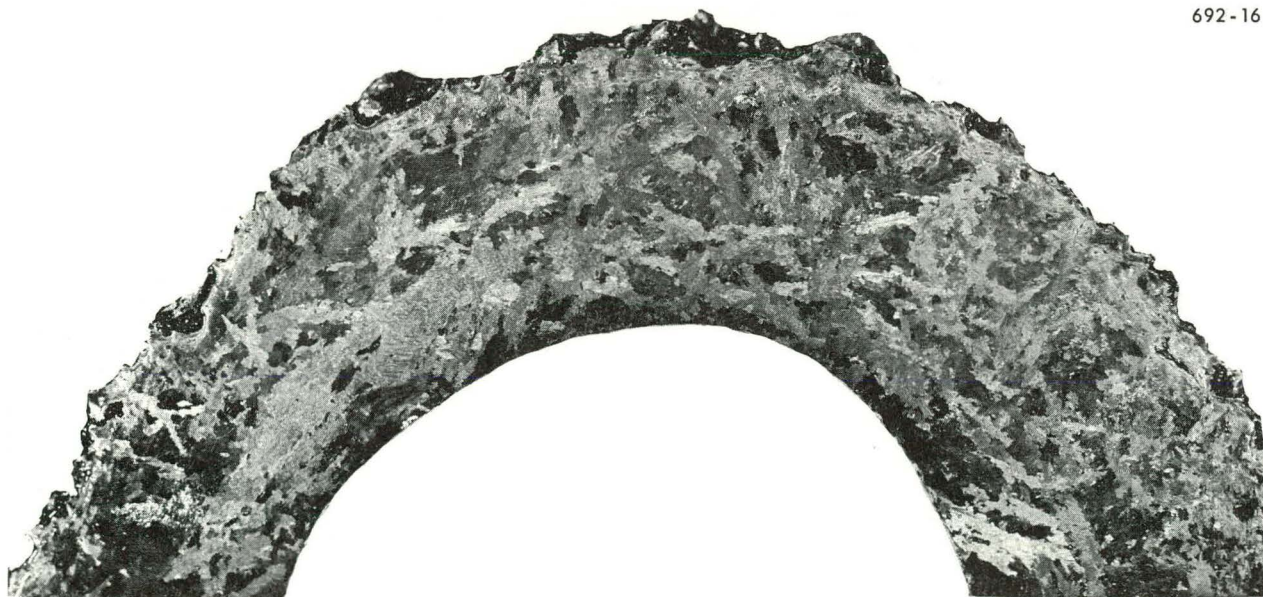
FIGURE 16 Rotary Elongated Tube, Roll Speed: 70 rpm; Beta-Phase Structure, Billet No. 33284 B3 (Rear), Tube No. 48, Transverse Section (3X)
