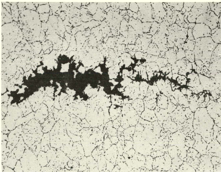
FIGURE A-5 TYPE 304 SS COLD WORKED EXPOSED TO CUPRIC CHLORIDE SOLUTION, 210-220 F, 20,000 PPM CHLORIDE, 1 HOUR OXALIC - ELECTROLYTIC ETCH
