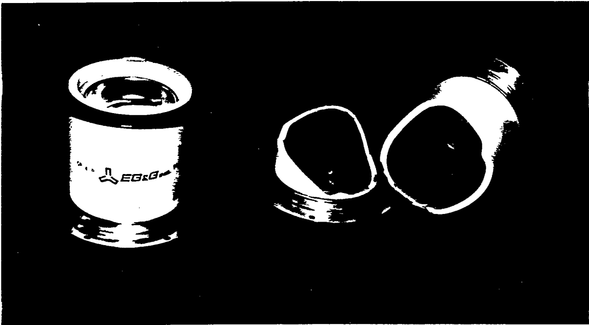
Figure 3-5 GP-41B Spark Gap Switch by EG&G a) original, b) damaged by internal breakdown
