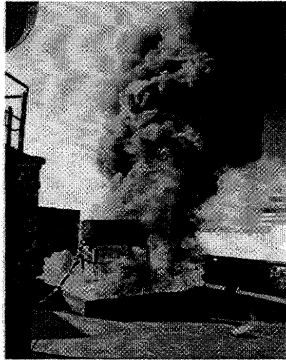
Figure 15. Diesel pool fire on deck of Mayo Lykes . In view at right, high wind has blown flames away from calorimeter.
