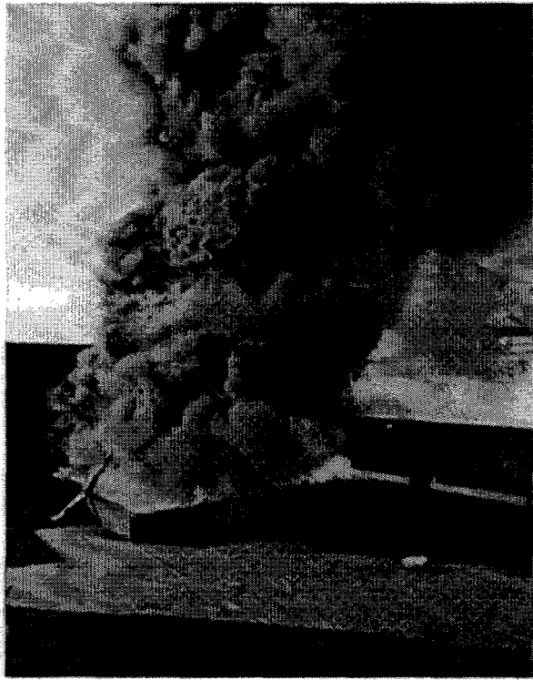
Figure 15. Diesel pool fire on deck of Mayo Lykes . In view at right, high wind has blown flames away from calorimeter.
