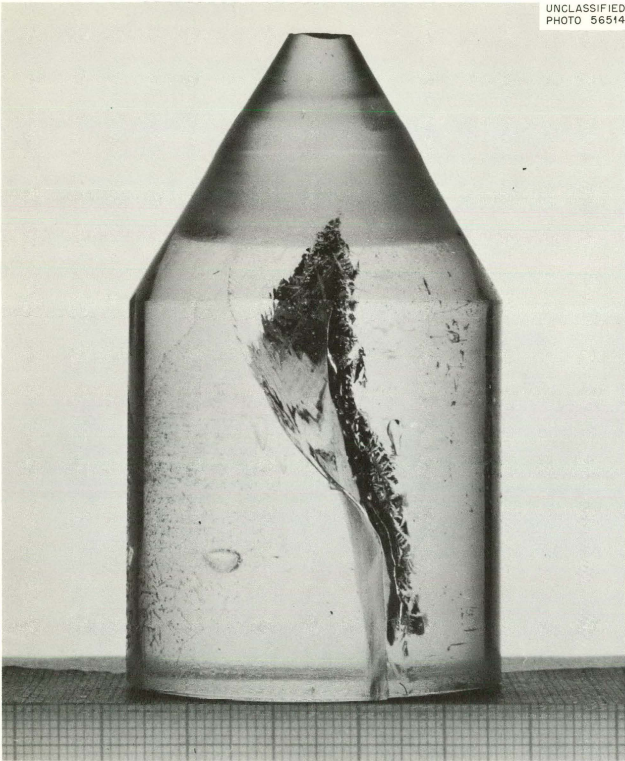
Fig. 34.1. Lithium Fluoride Bicrystal Which Weighed 300 g (Showing Minor Bubble Formation).
