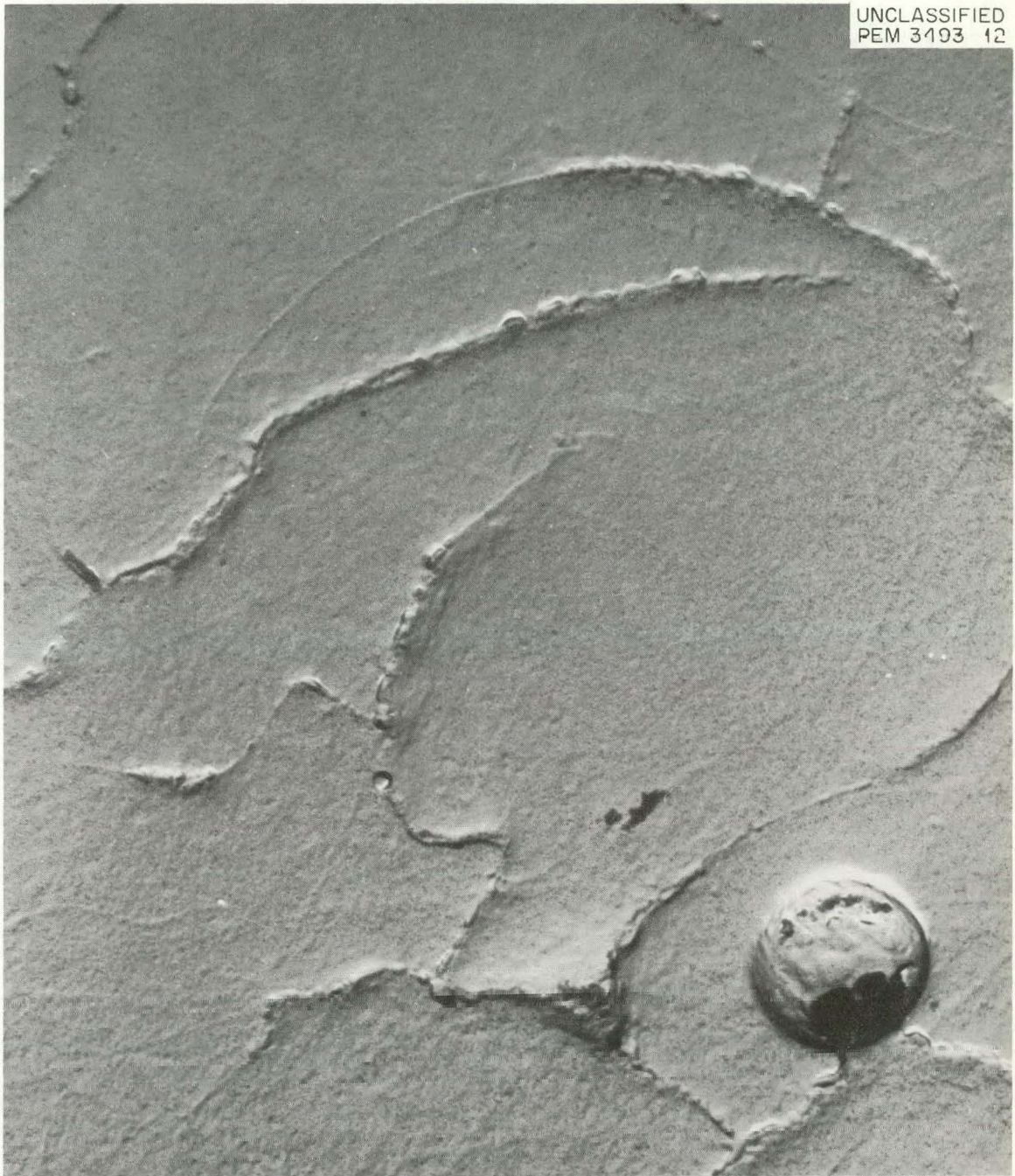
Fig. 14.6. Photomicrograph: 90 mole % Urania Specimen Heated at 291°C. 20,000X. Reduced 14.5%.
