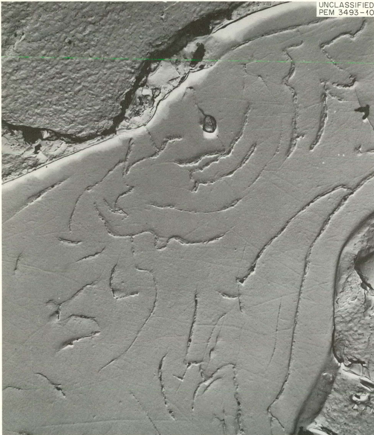
Fig. 14.5. Photomicrograph: 90 mole % Urania Specimen Heated at 291°C. 8000X. Reduced 7%.
