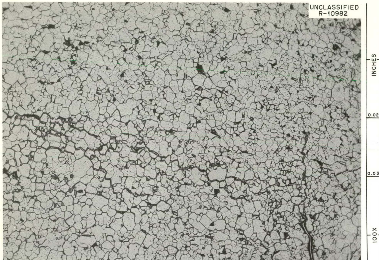
Fig. 19.7. Photomicrograph of Irradiated Cold-Pressed and Sintered BeO Specimen 7-5-2 Exposed to 3.65 \times 10^{21} nvt ( > 1 Mev) at 926^\circ\text{C} in Experiment 41-7 (As Polished, 100X).
