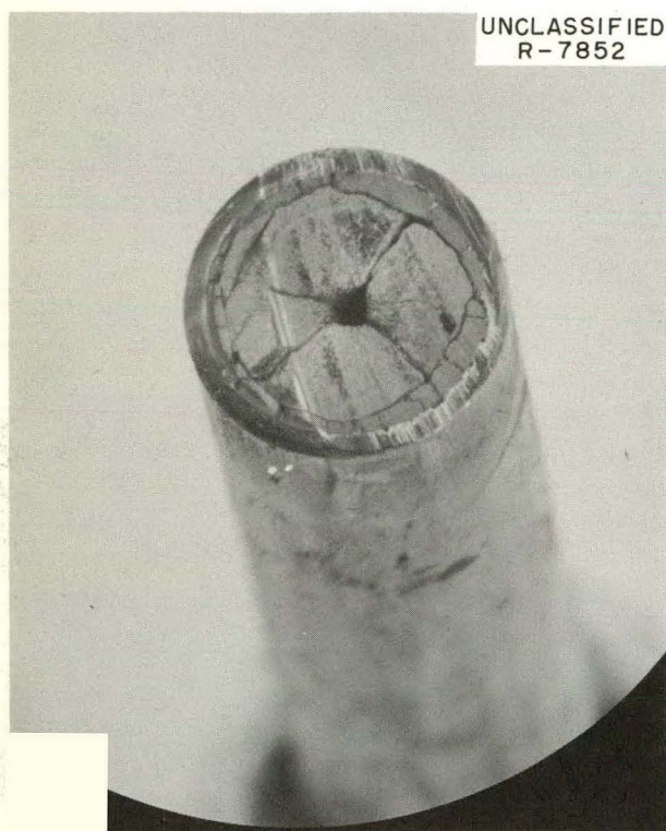
Fig. 20.1. Cross Section of Capsule 06-4, Showing a Central Void in the \text{UO}_2 .
