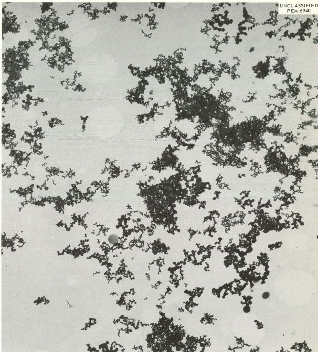
Fig. 23.3. \text{UO}_2 Particles Collected on the Millipore Filter Paper. 26,000X.
