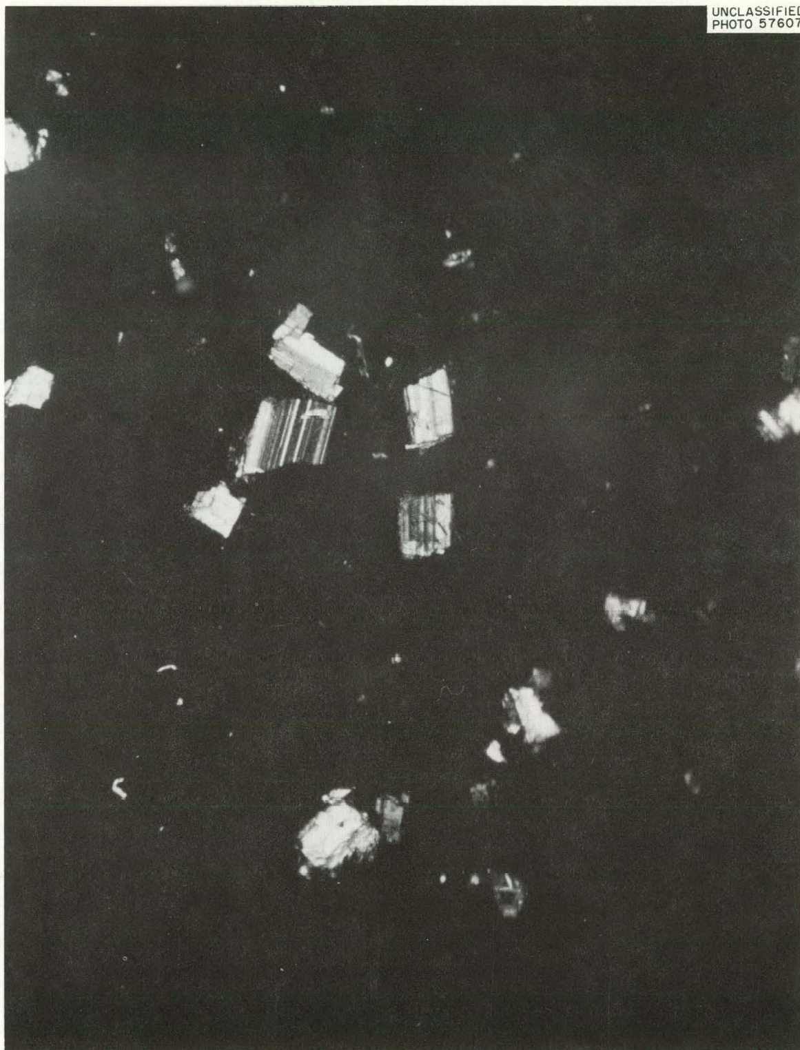
Fig. 1.5. Photomicrograph of Multiply Twinned \text{LiCsF}_2
