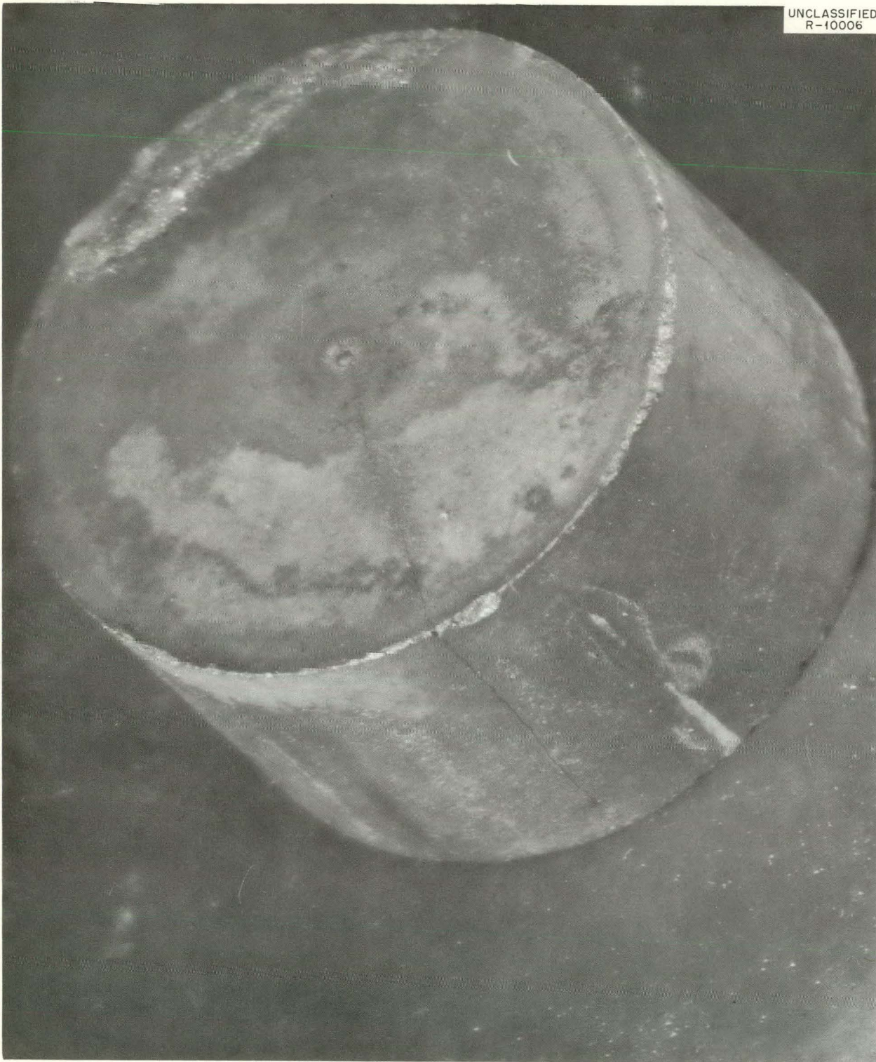
Fig. 19.2. Typical Fractured Pellet, ORNL Experiment 41-7, Specimen 7-4-4.
