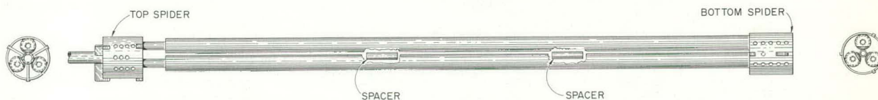
Fig. 20.7. Schematic of Experimental Fuel-Rod Bundle, Maritime Reactor Program.
