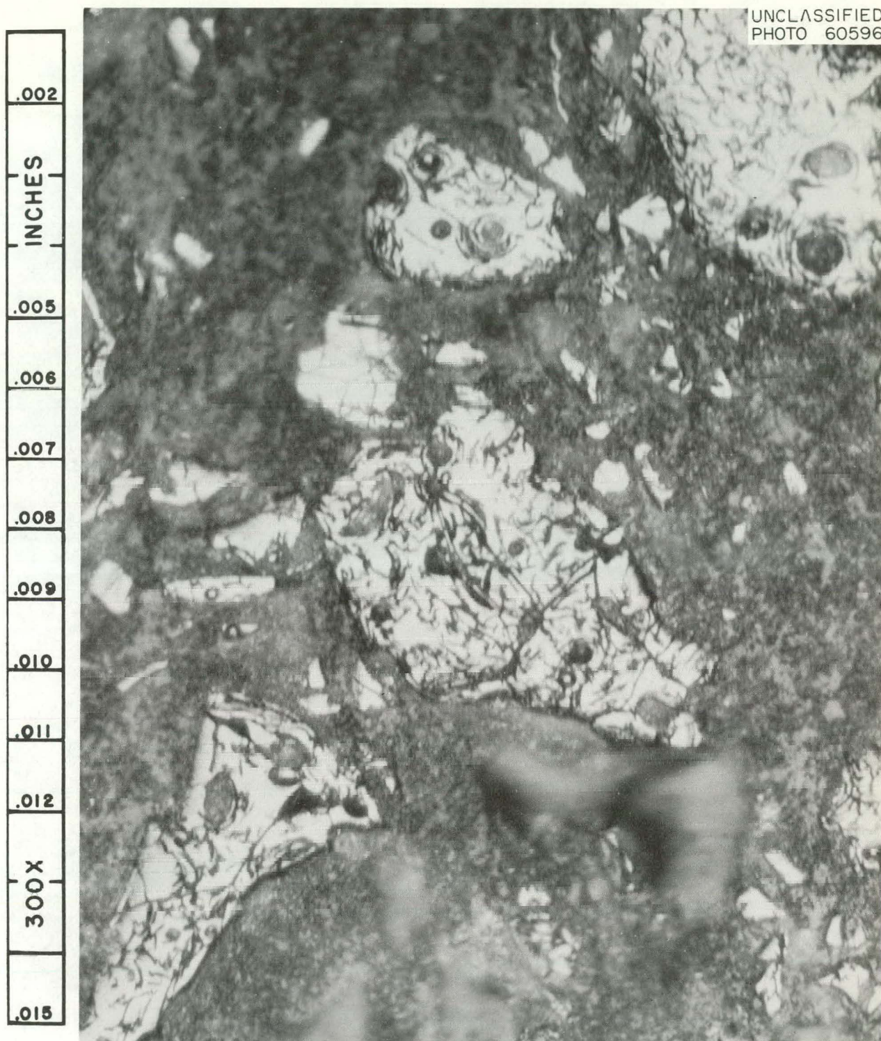
Fig. 14.4. Photomicrograph: 90 mole % Urania Specimen Heated at 291°C. 300X. Reduced 8%.
