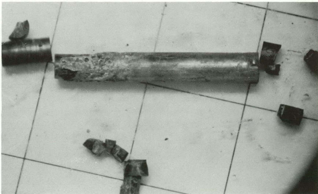
Fig. 21. Partially-dissolved Zircaloy-2-clad Mark I specimen irradiated in NTX to 16,800 Mwd/ton. (Background is 1-inch grid.)
