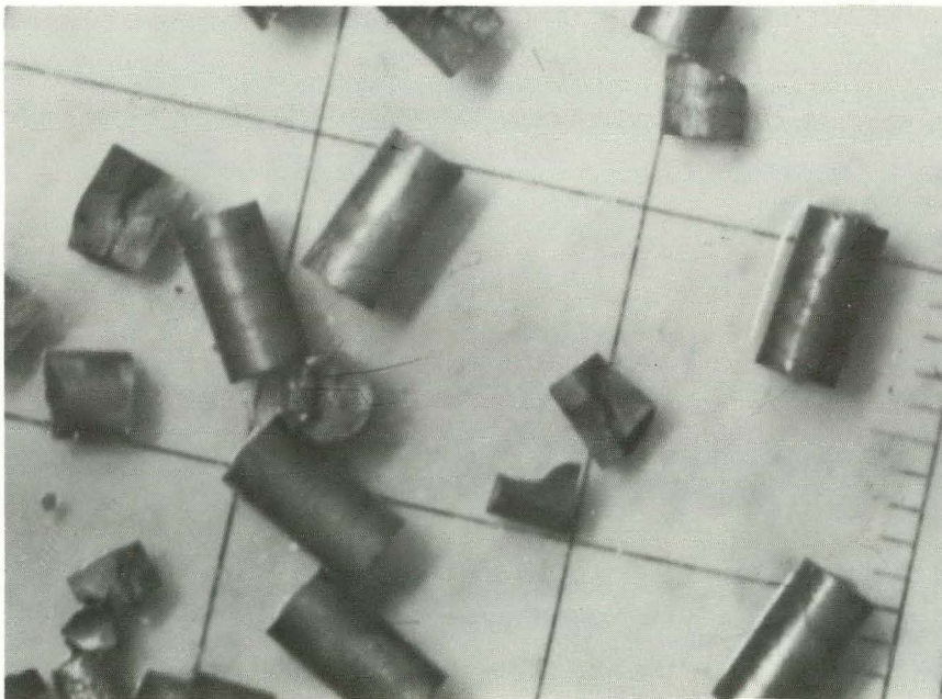
Fig. 36. \text{UO}_2 pellets from HZ-19 on 1-in. grid. Numec (NRX) pellets irradiated to 14,600 Mwd/ton U.
