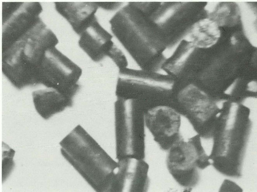
Fig. 38. \text{UO}_2 pellets from HS 23-24 in 3-in. pan. Numec pellets irradiated to 25,600 Mwd/ton in NRX reactor.
