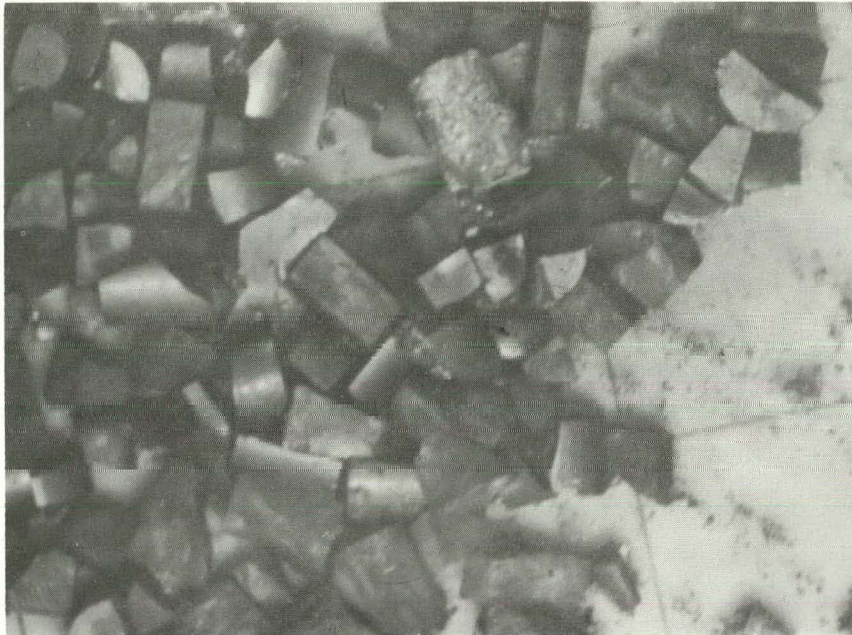
Fig. 29. \text{UO}_2 pellets from HZ-22 on 1-in. grid. WAPD-PWR rod irradiated to 6156 Mwd/ton U.
