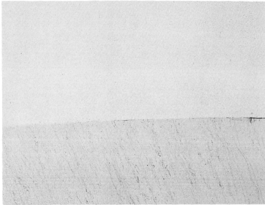
FIGURE 18 - Photomicrograph of liner-strength member interface. Unetched, 130X
