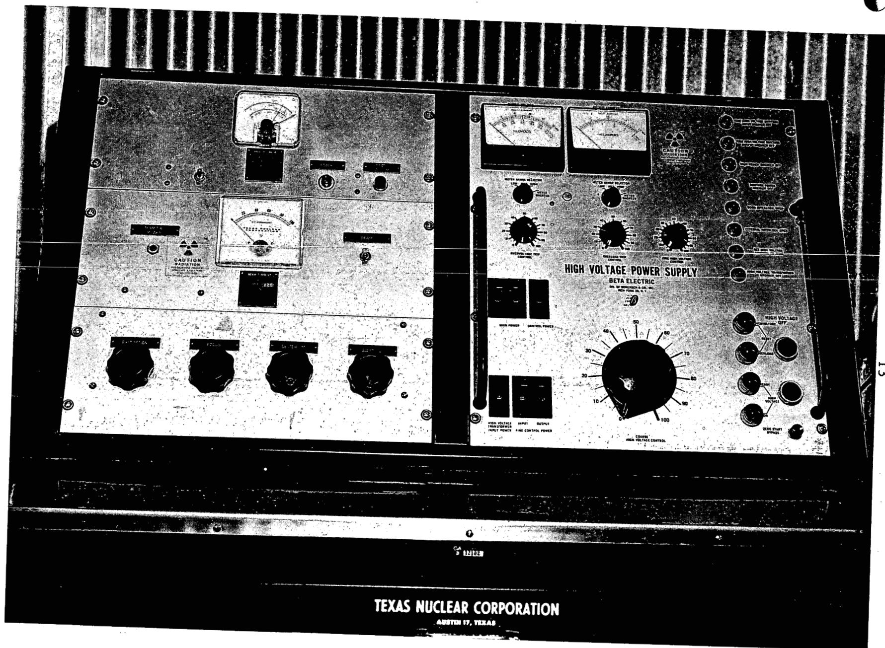
Fig. 7--Control console for neutron generator
