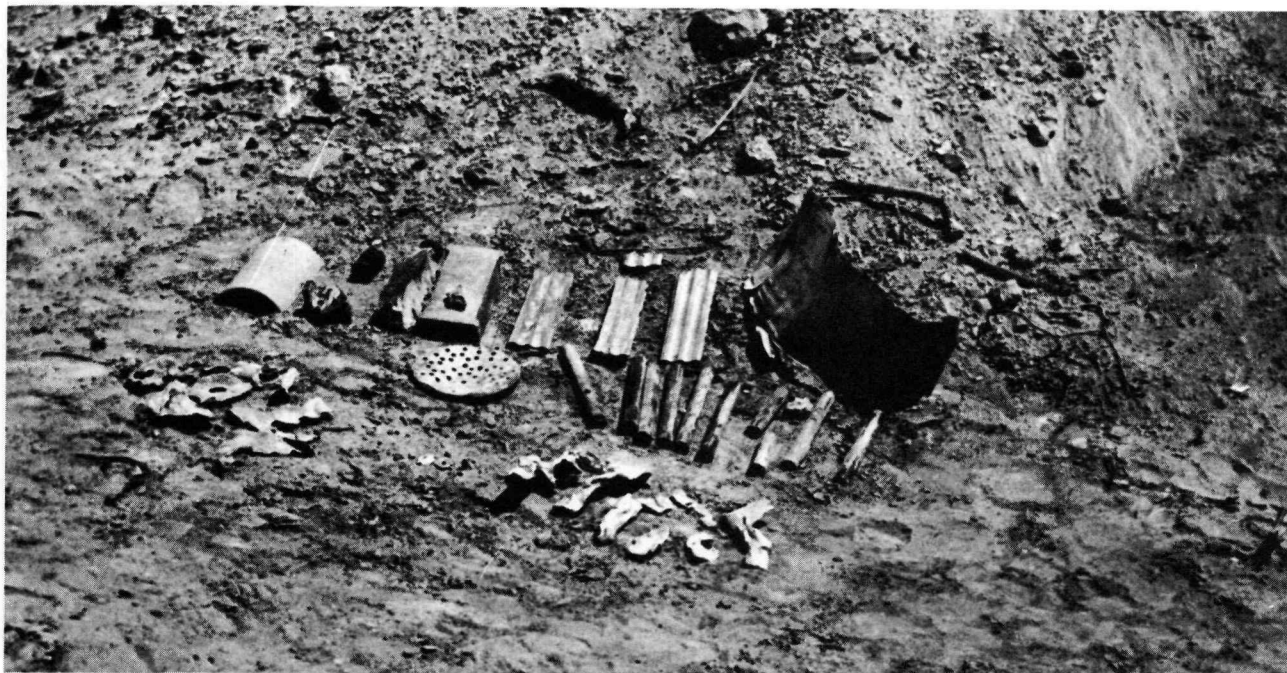
Figure 6. Test Article After Concrete Impact
