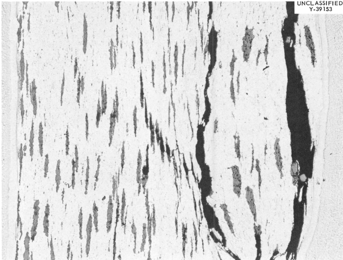
Fig. 11. Transverse Cross Section of a Zr-3 wt % Al-Clad Plate Showing Large Cracks in the Core and a Diffusion Layer Extending into the Cladding (Plate 4 of Table 13). As-polished. 100X.
