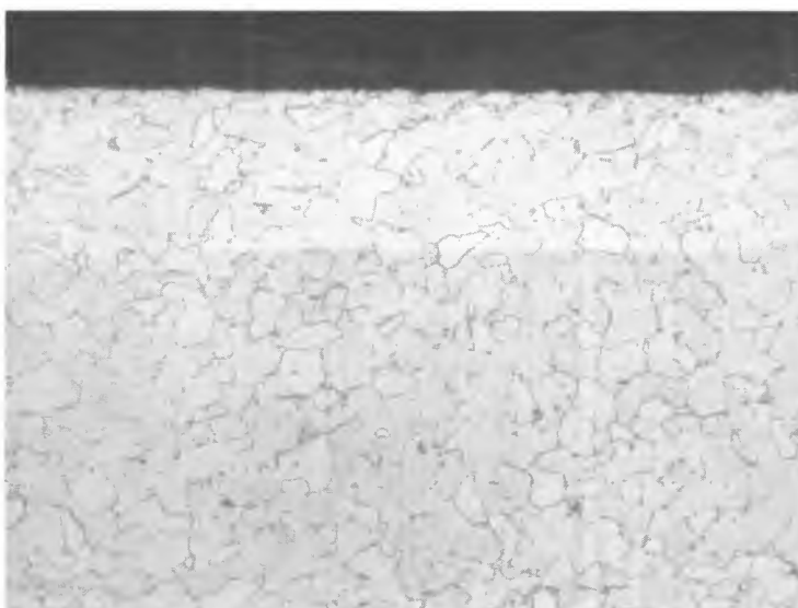
FIG 25 - 2 1/4 Cr-1 Mo #2ALX4 Creep in 1100°F Sodium
