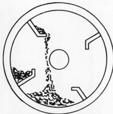
ROTARY CAGE FOR COATING POWDERS FIGURE 1
