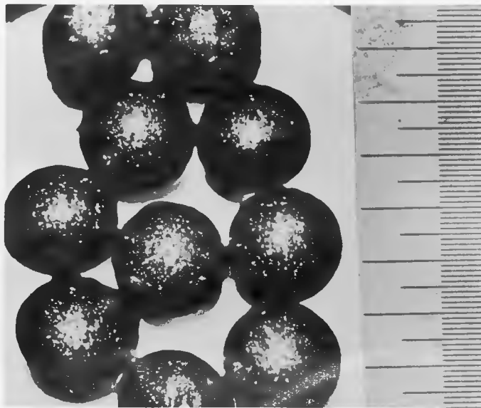
Fig. 1 Spheric \text{UO}_2 particles 100 x
