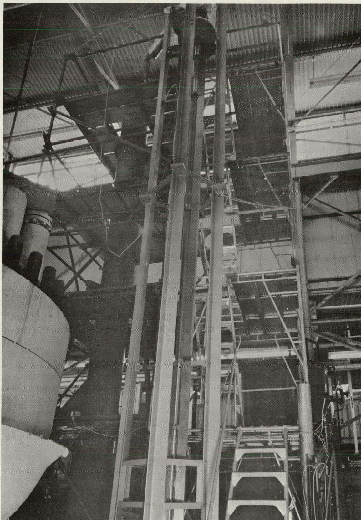
Fig. 1.02...Oscillator Rod Internals on Test Assembly (7D-0-2)
