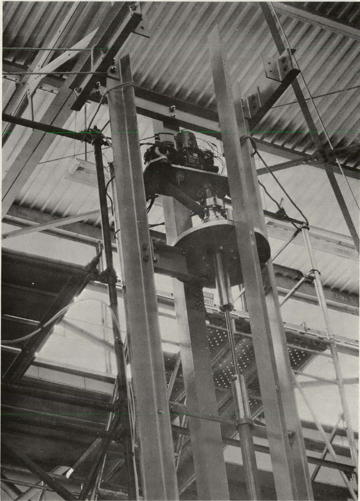
Fig. 1.03...Oscillator Rod Drive Unit on Test Assembly (7D-0-3)
