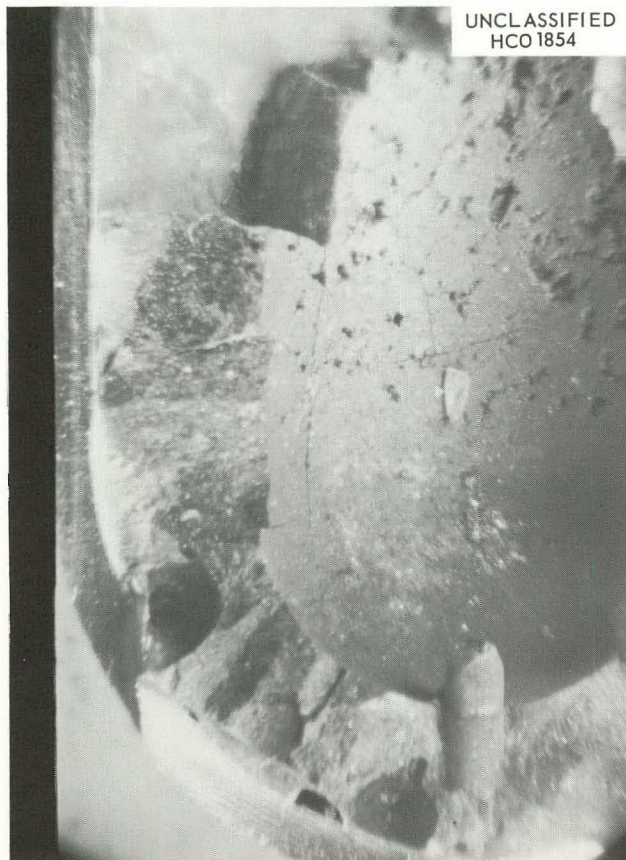
Fig. 5.4. Bubbles Near Bottom of Capsule 12. The graphite core was removed before this photograph was taken. There were no bubbles on the sides of the capsule.
