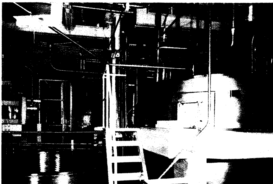
Fig. 36. Vessels used for plutonium purification and concentration.
