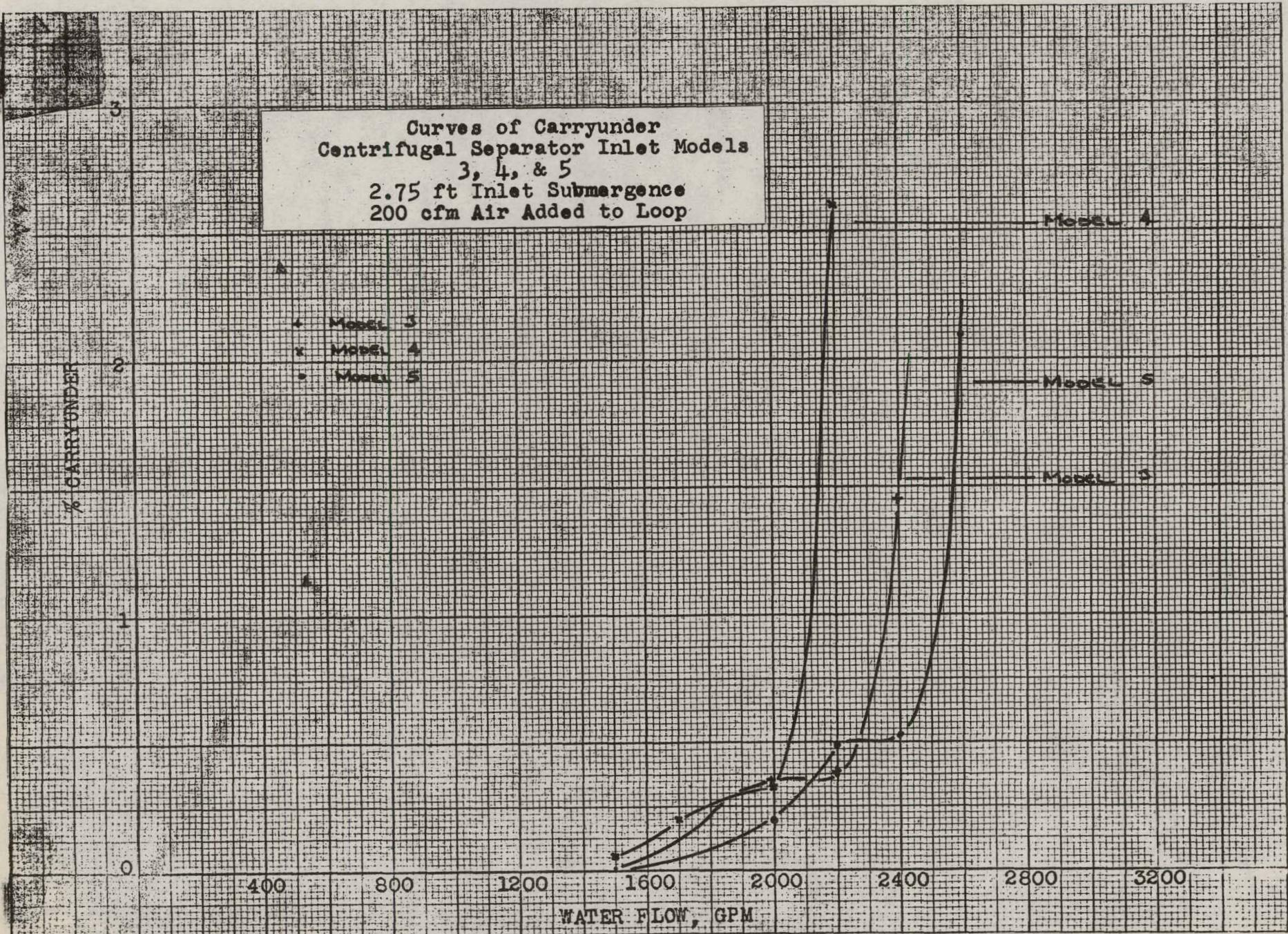
Figure 44 - Carryunder for Separator Inlets 3, 4 and 5
