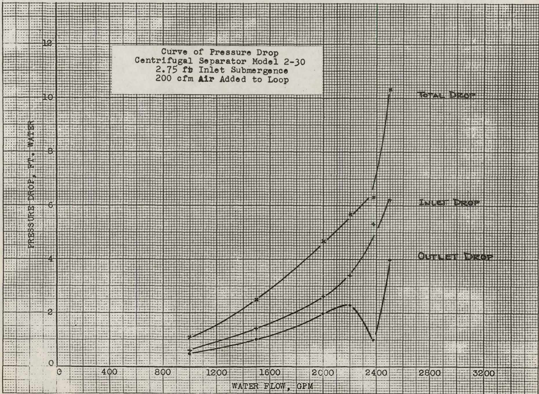
Figure 24 - Performance Curves for Separator Model 2-30
