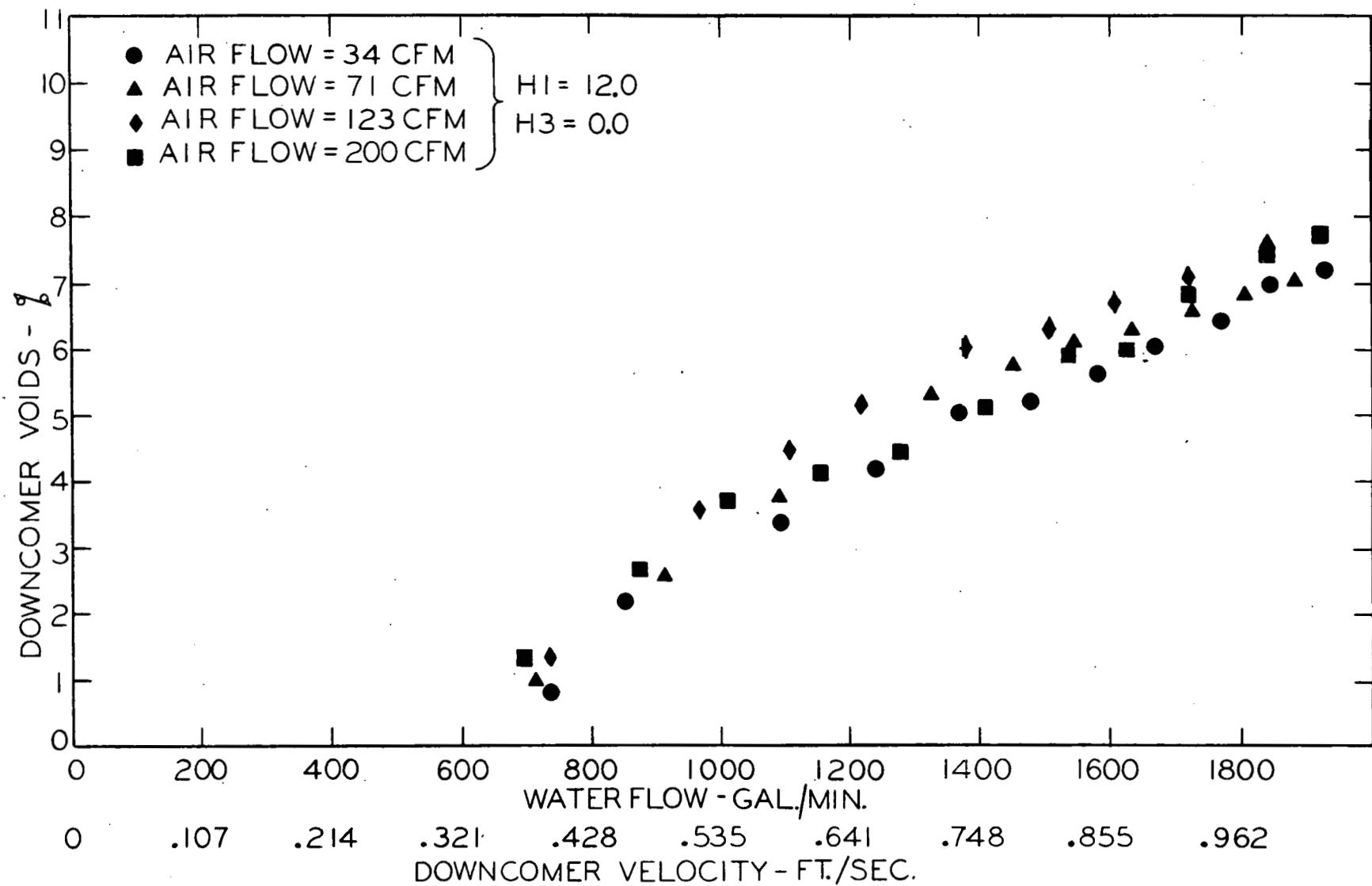
Figure 6 - Effect of Air Flow on Downcomer Voids (Loop Temp.  $150^{\circ}\text{F} \pm 3^{\circ}$ )
