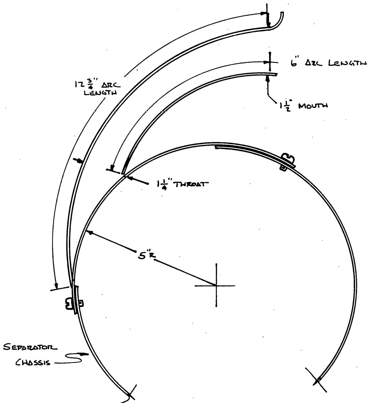
Figure 32 - Inlet Nozzle Model 2
