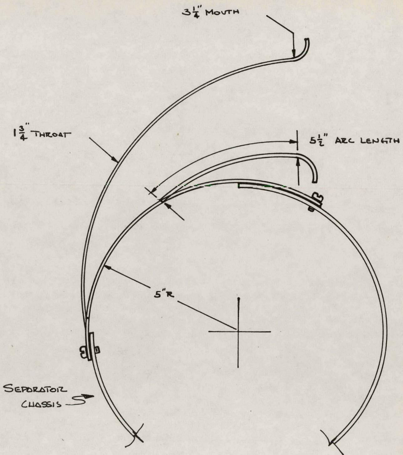
Figure 38 - Inlet Nozzle Model 5
