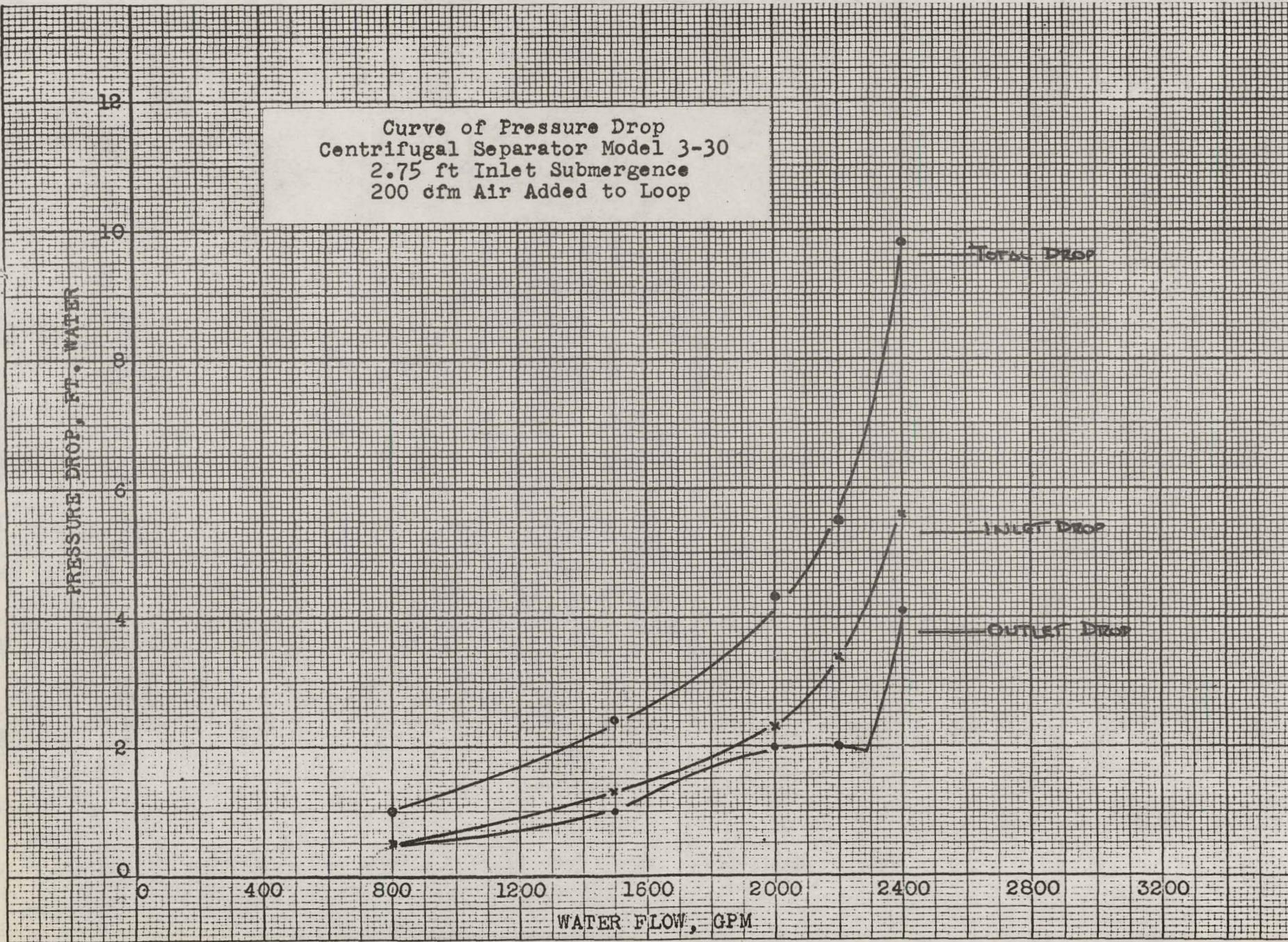
Figure 41 - Performance of Separator Model 3-30
