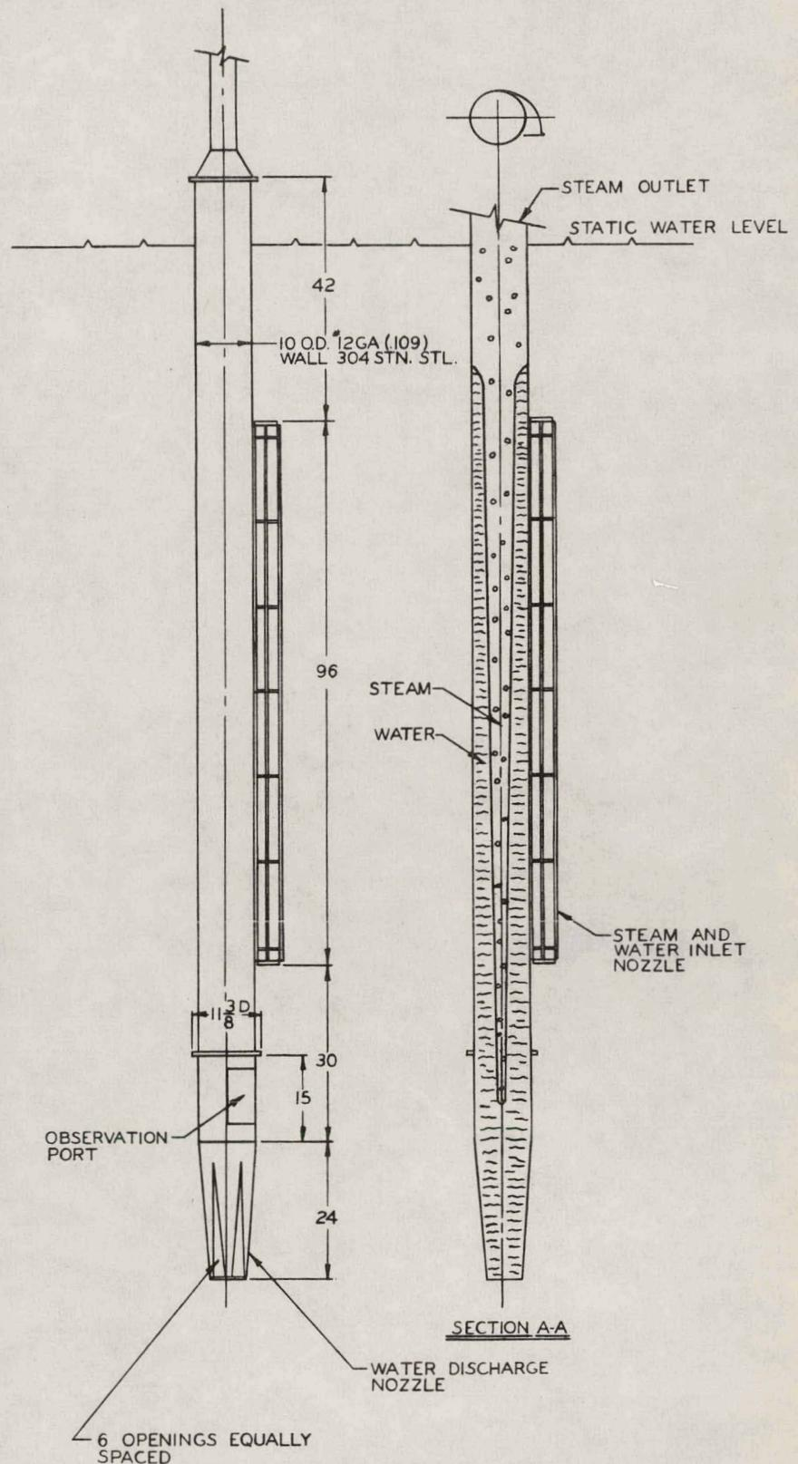
Figure 19 - Ten Inch Diameter Centrifugal Steam Separator Model
