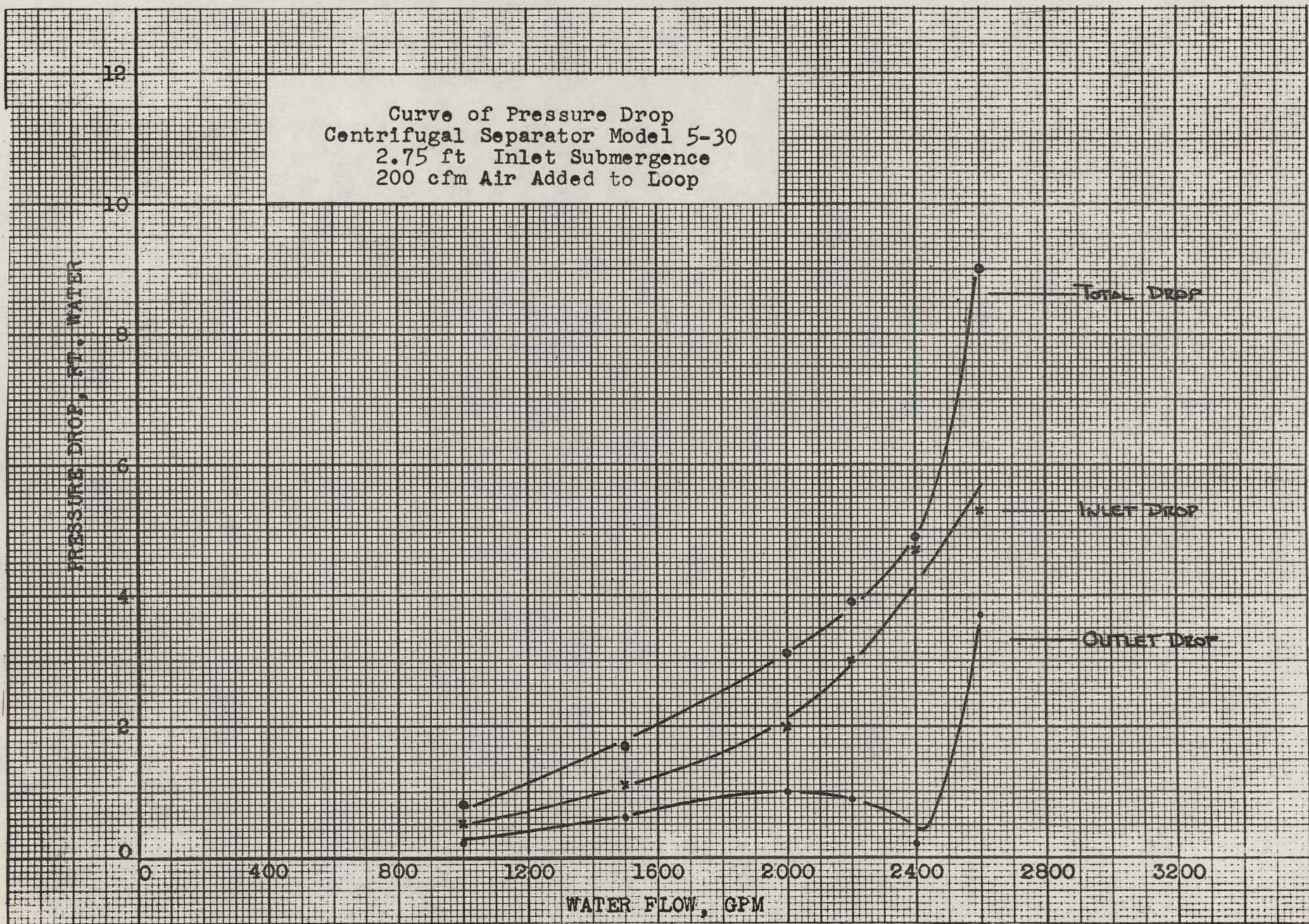
Figure 43 - Performance of Separator Model 5-30
