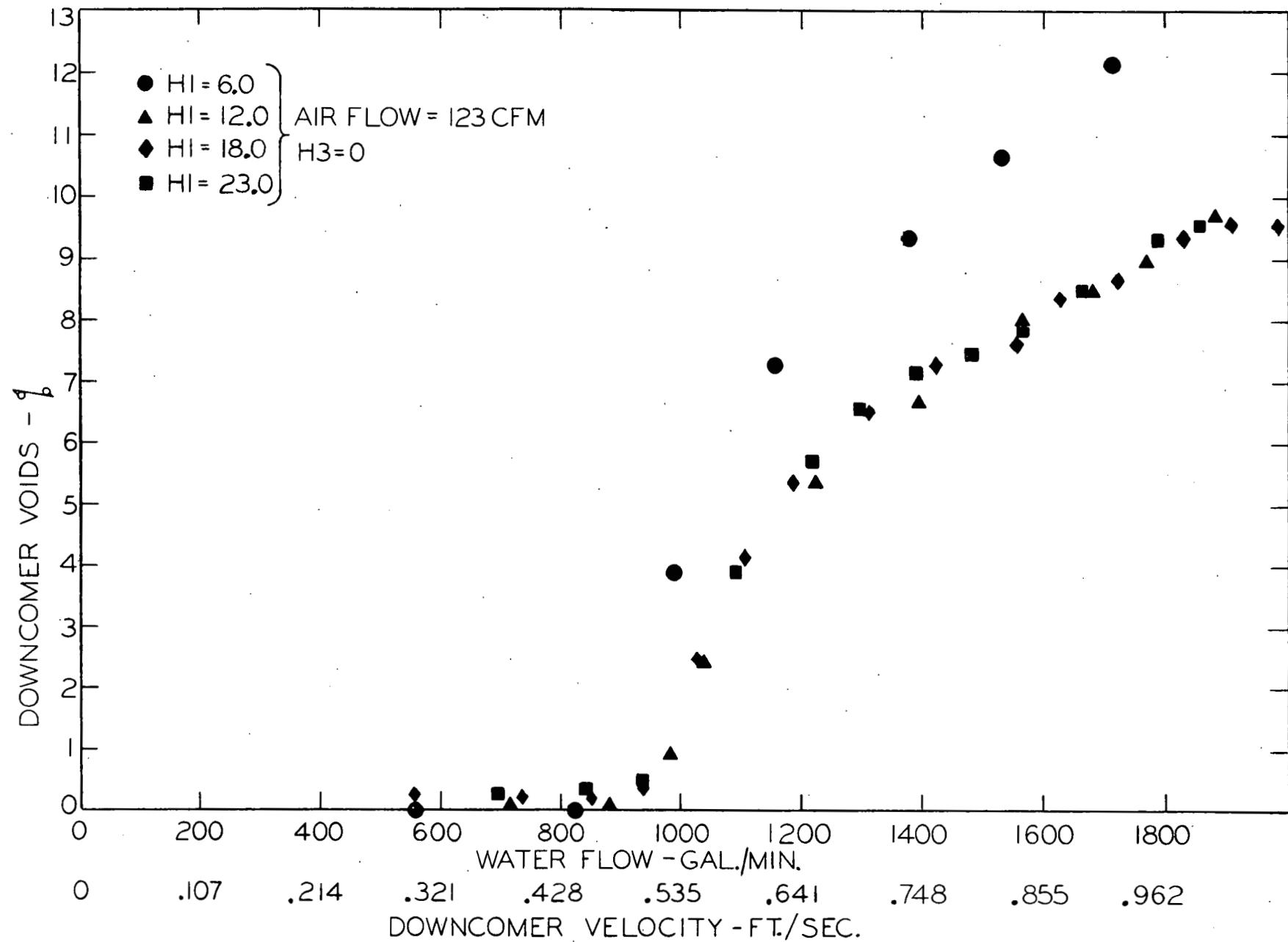
Figure 7 - Effect of Riser Length on Downcomer Voids (Loop Temp.  $90^{\circ}\text{F} \pm 5^{\circ}$ )
