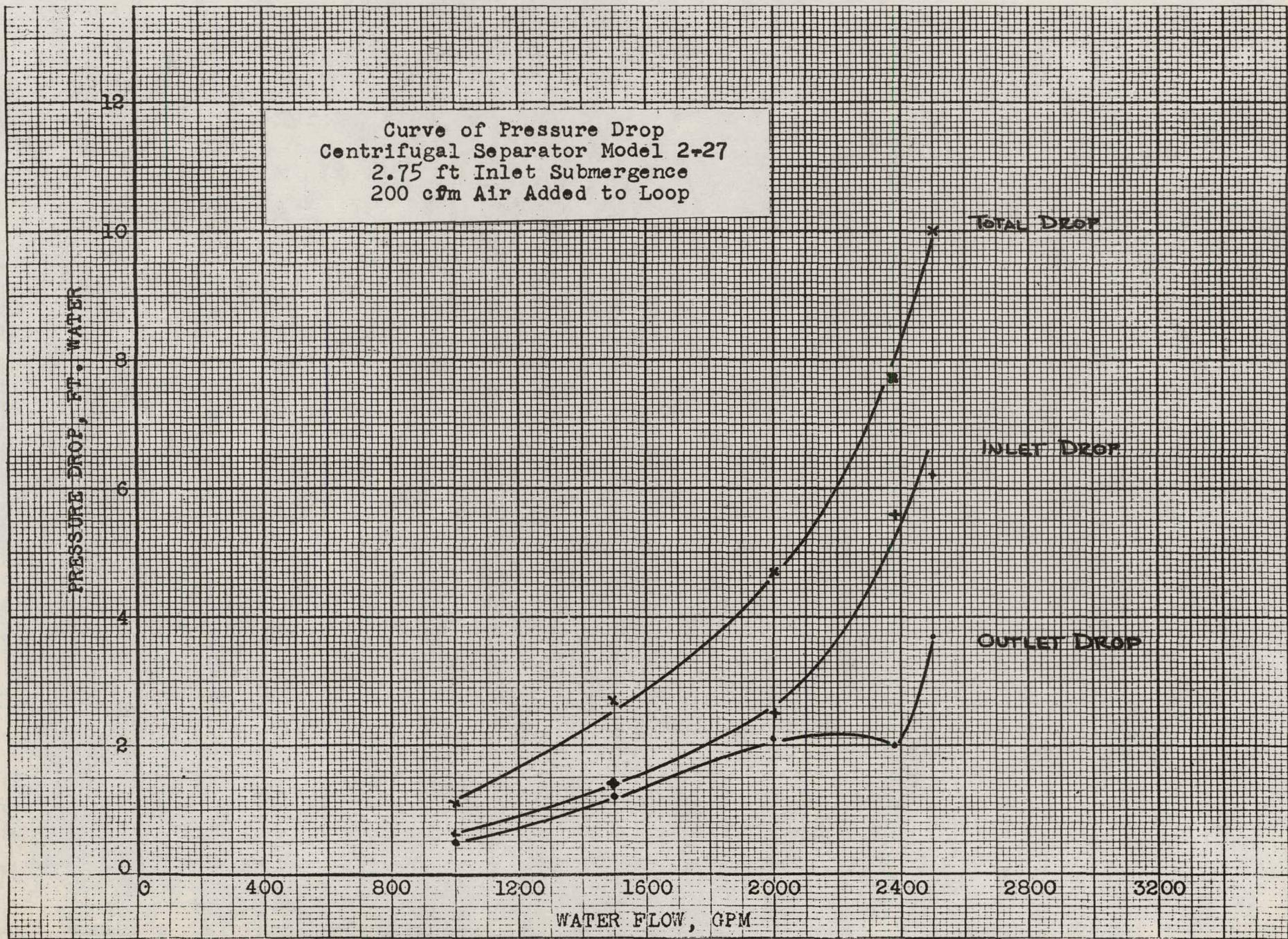
Figure 22 - Performance Curves for Separator Model 2-27
