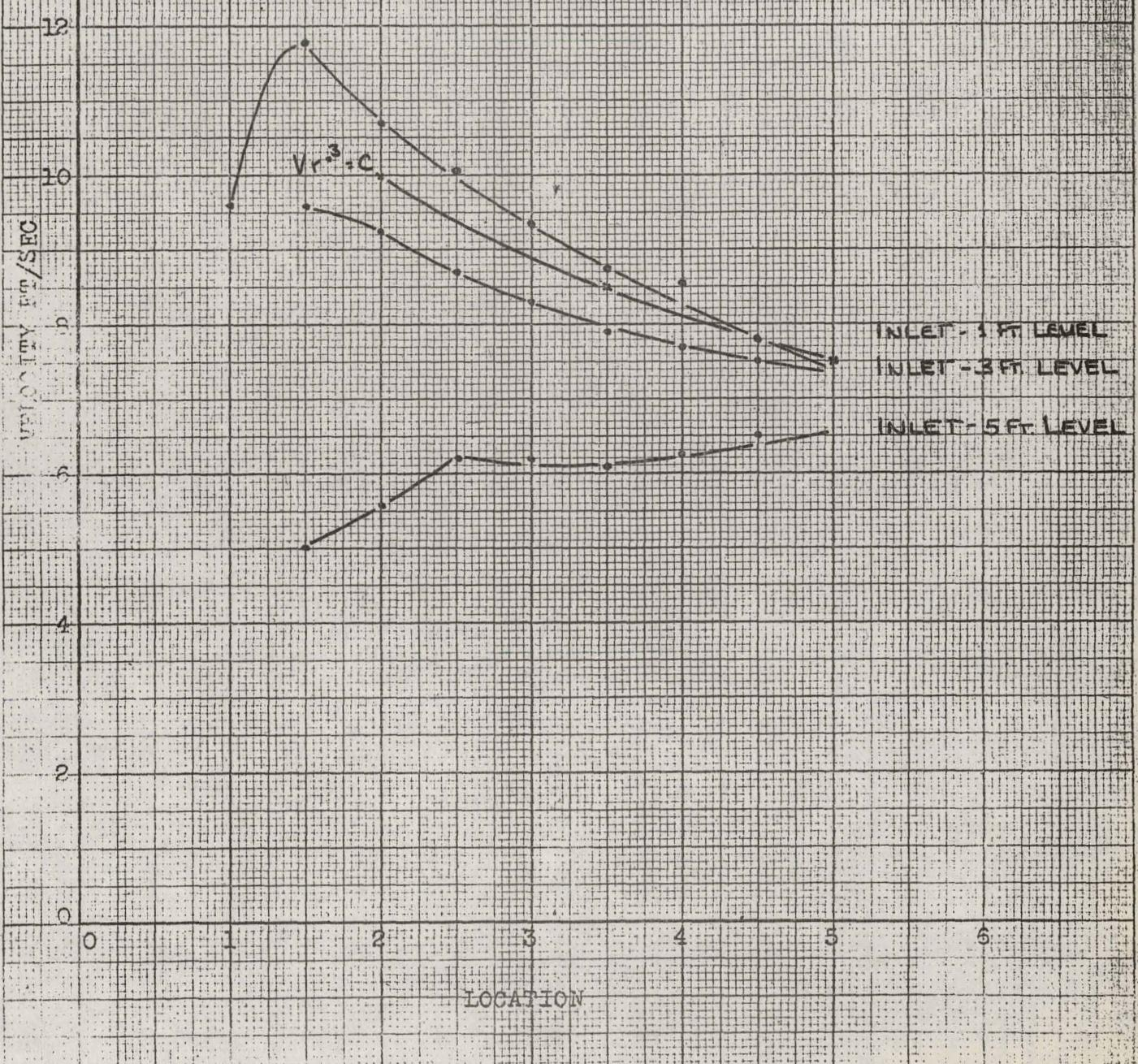
Figure 35 - Velocity Profile of Model 3 Inlet Nozzle
