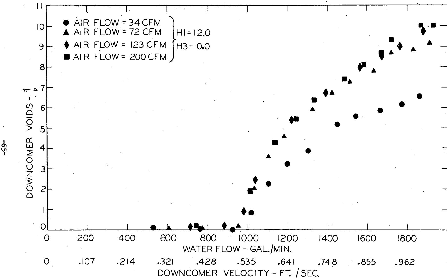
Figure 5 - Effect of Air Flow on Downcomer Voids (Loop Temp.  $90^{\circ}\text{F} \pm 6^{\circ}$ )
