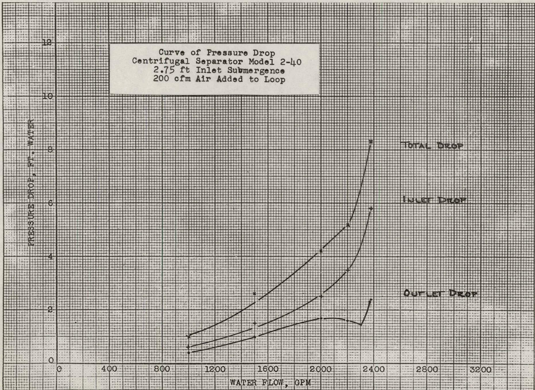
Figure 28 - Performance Curves for Separator Model 2-40
