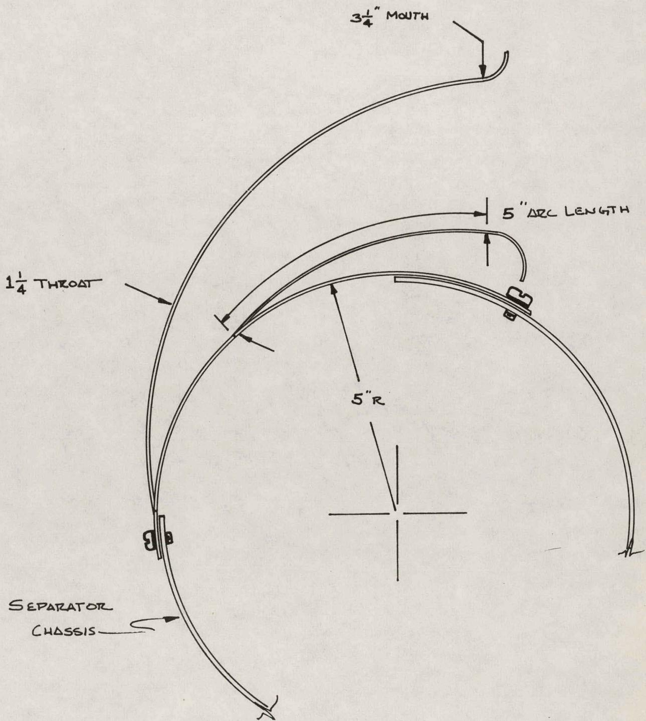
Figure 34 - Inlet Nozzle Model 3
