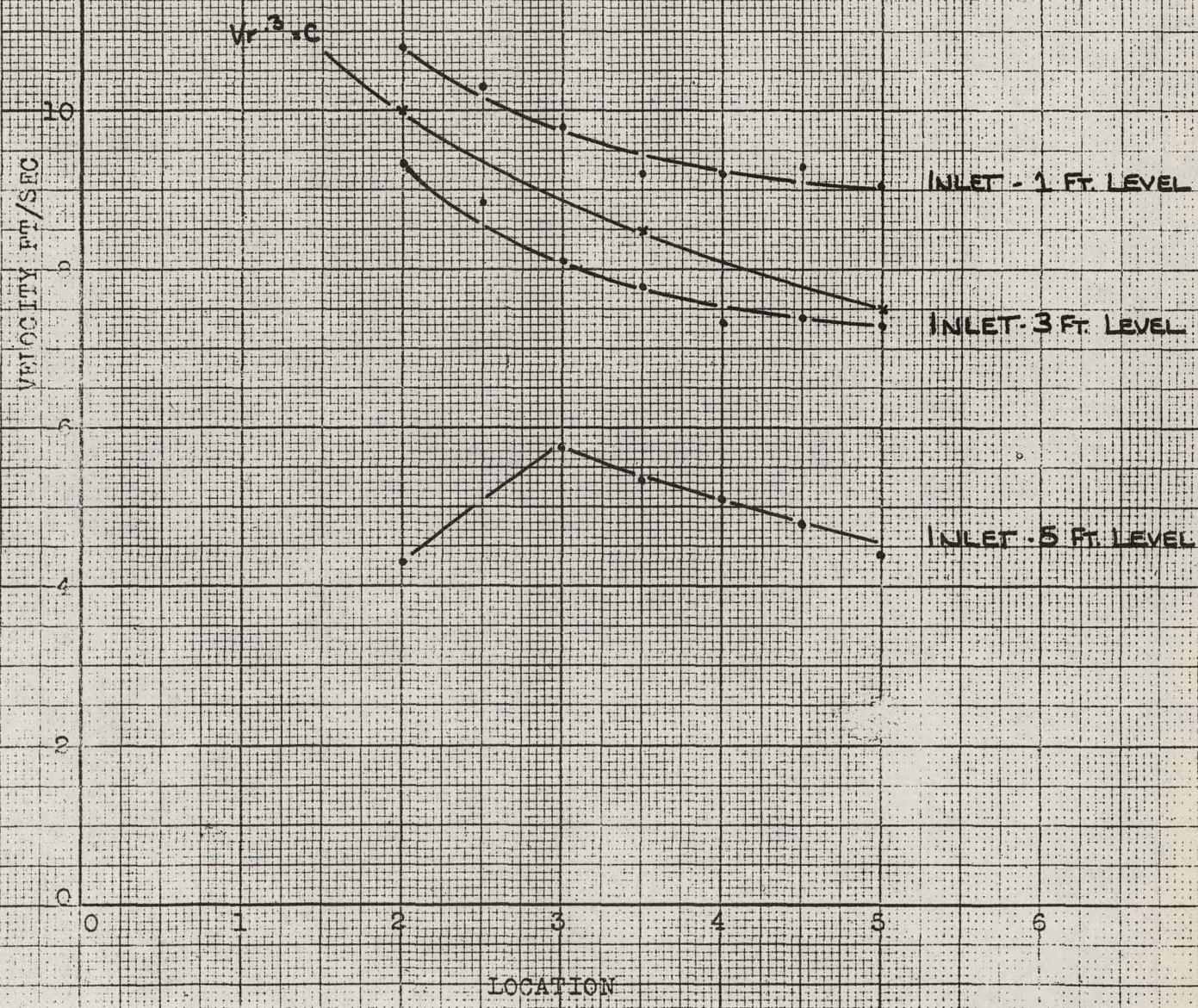
Figure 33 - Velocity Profile of Model 2 Inlet Nozzle
