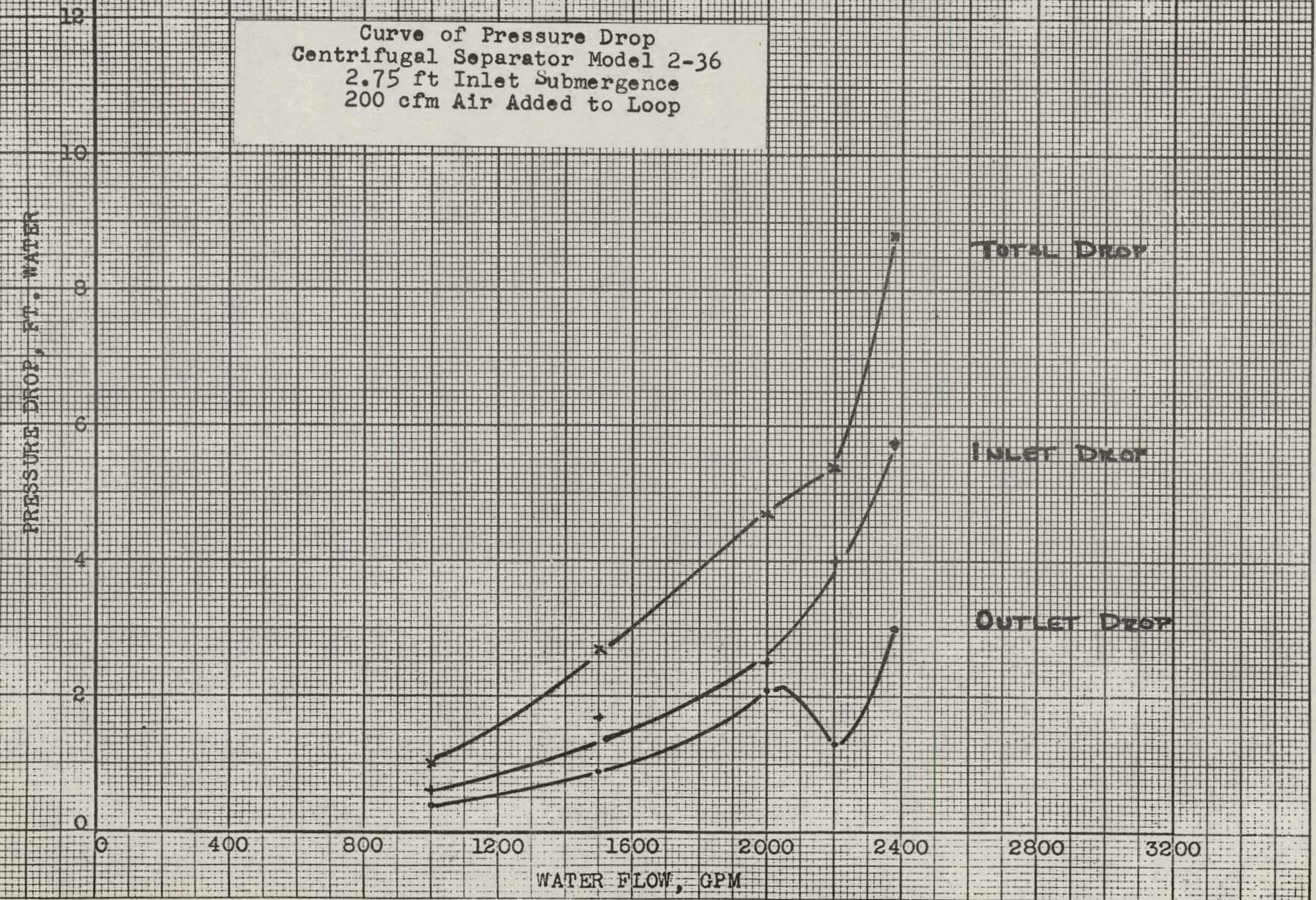
Figure 27 - Performance Curves for Separator Model 2-36
