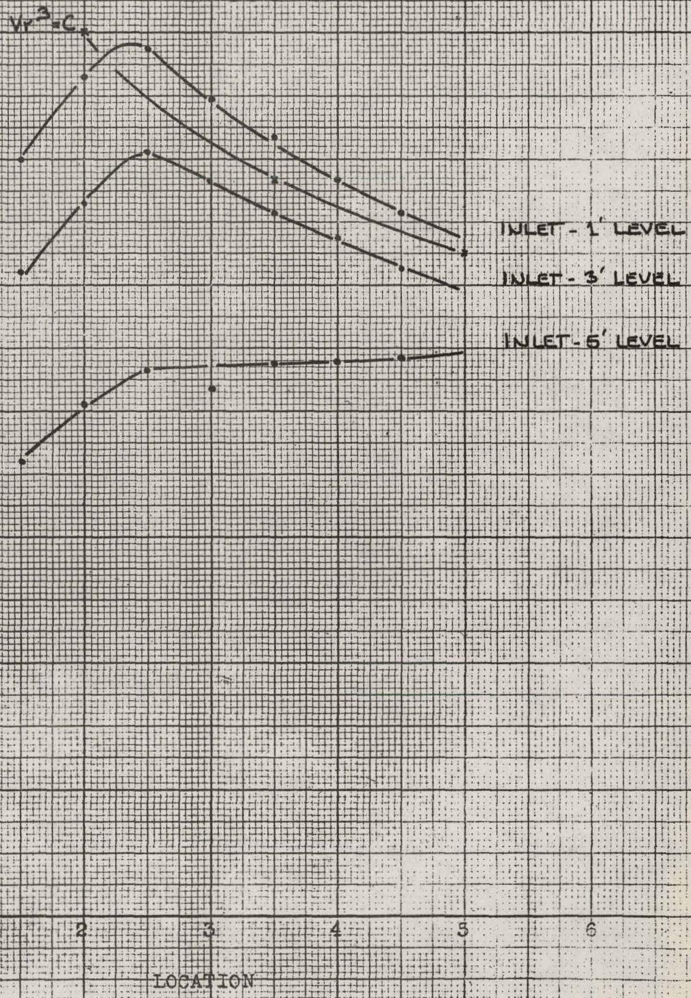
Figure 37 - Velocity Profile of Model 4 Inlet Nozzle
