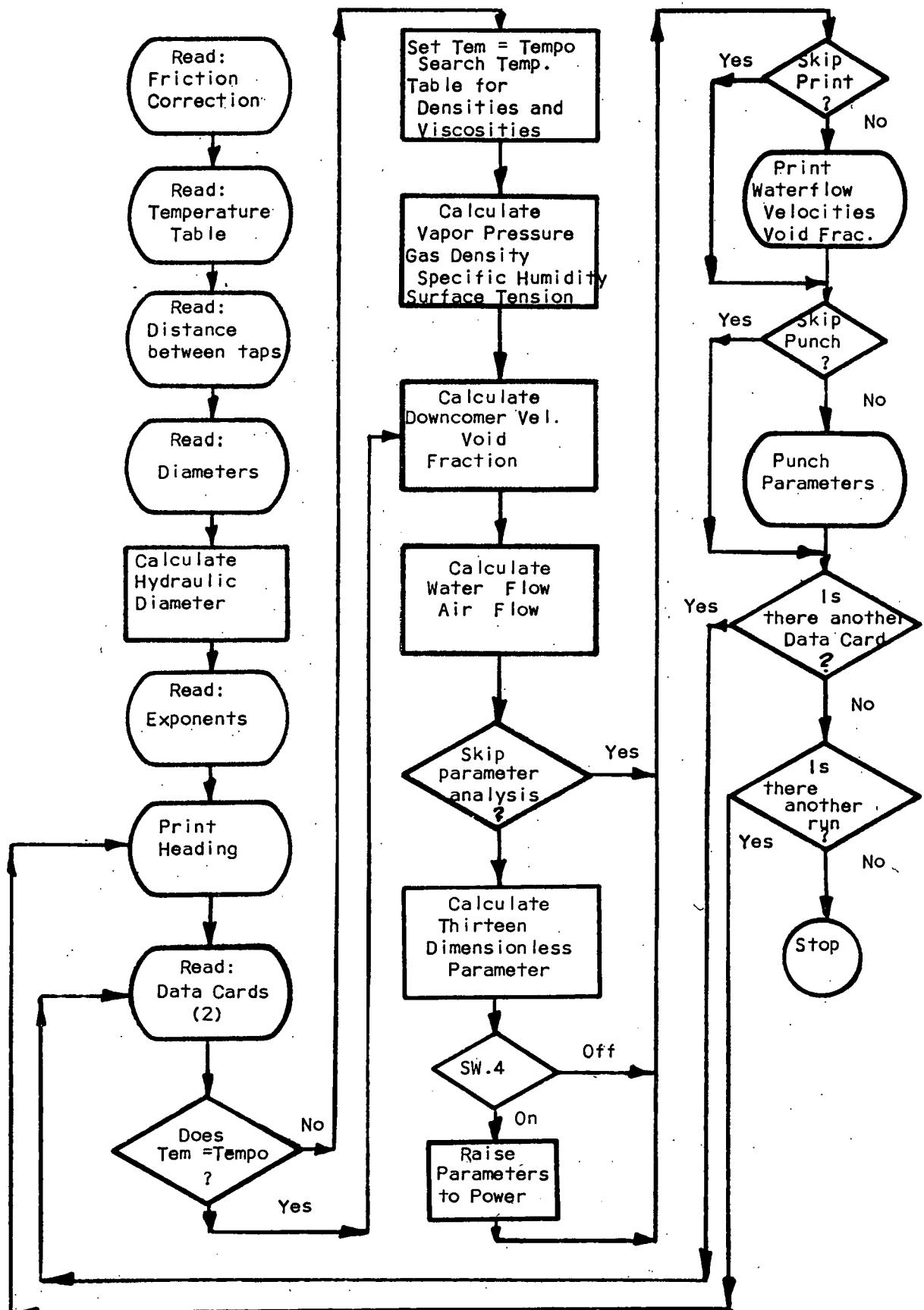
Figure 3 - Air-Water Tank Data Reduction Logic Program
