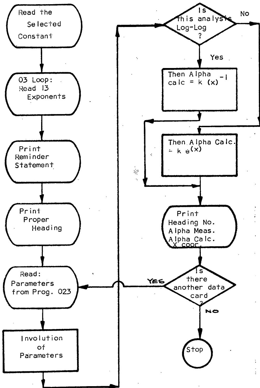
Figure 16 - Logic Diagram for Program 25
