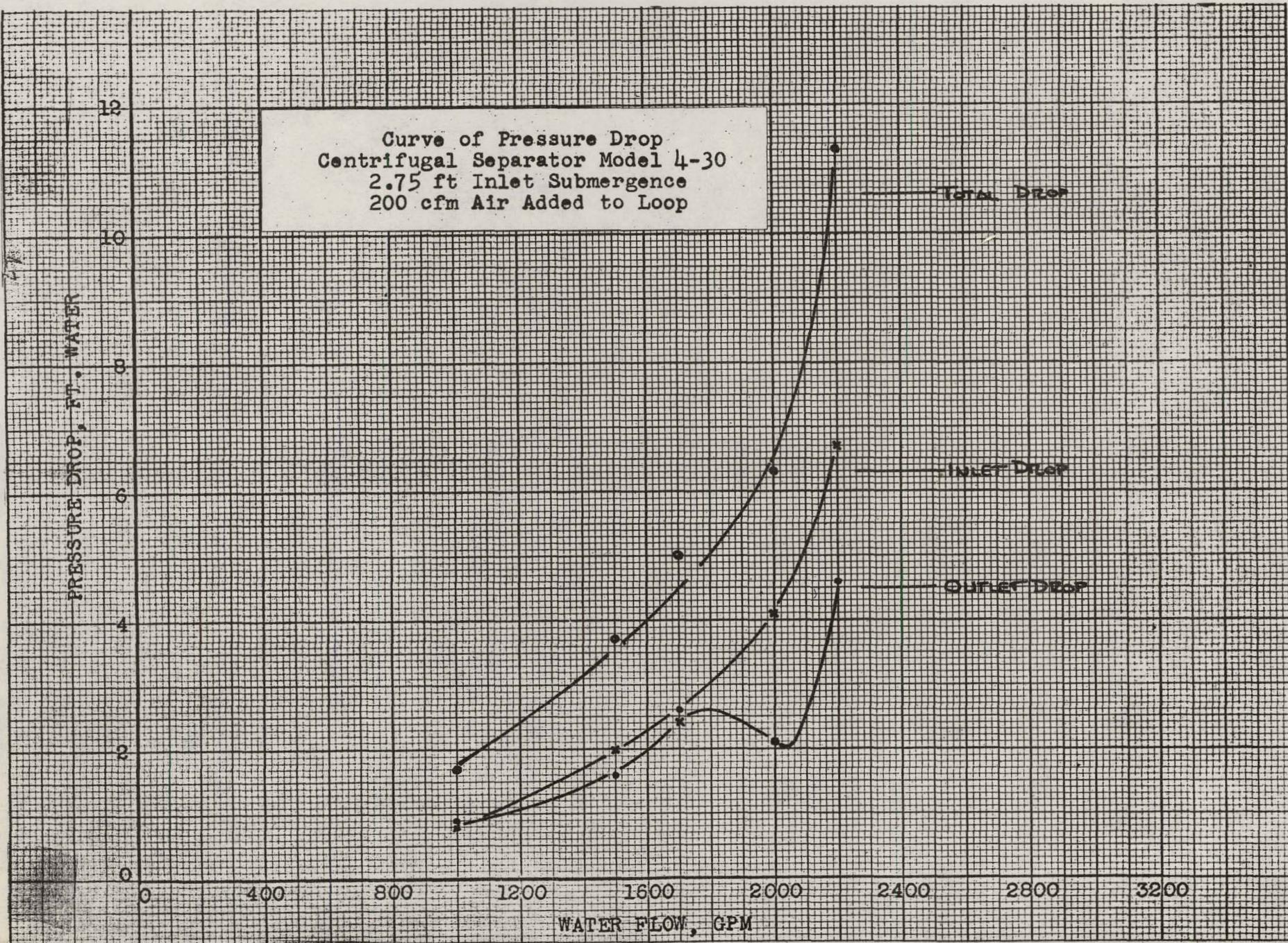
Figure 42 - Performance of Separator Model 4-30
