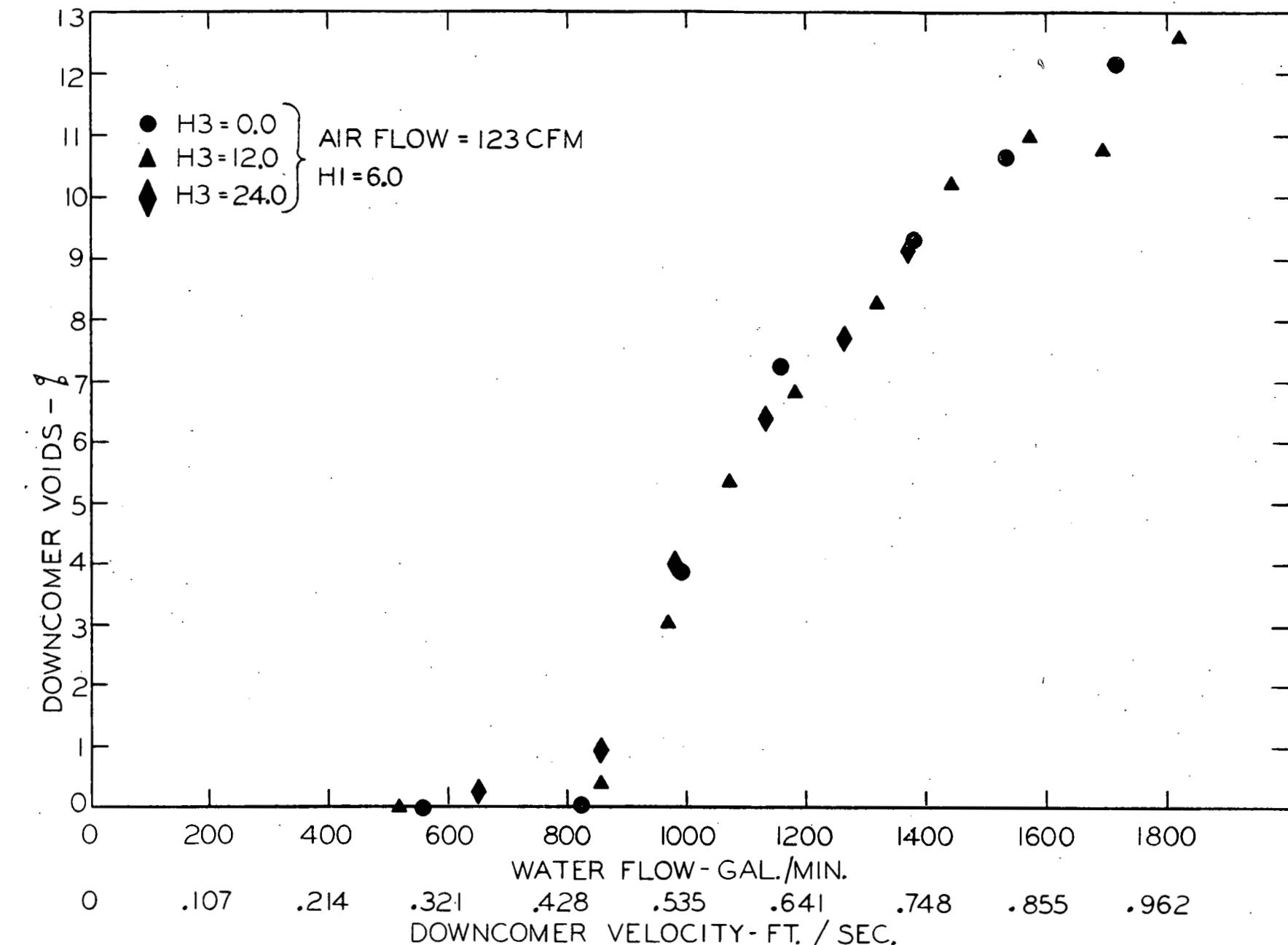
Figure 9 - Effect of Initial Water Level on Downcomer Voids (Loop Temp.,  $90^{\circ}\text{F} \pm 5^{\circ}$ )
