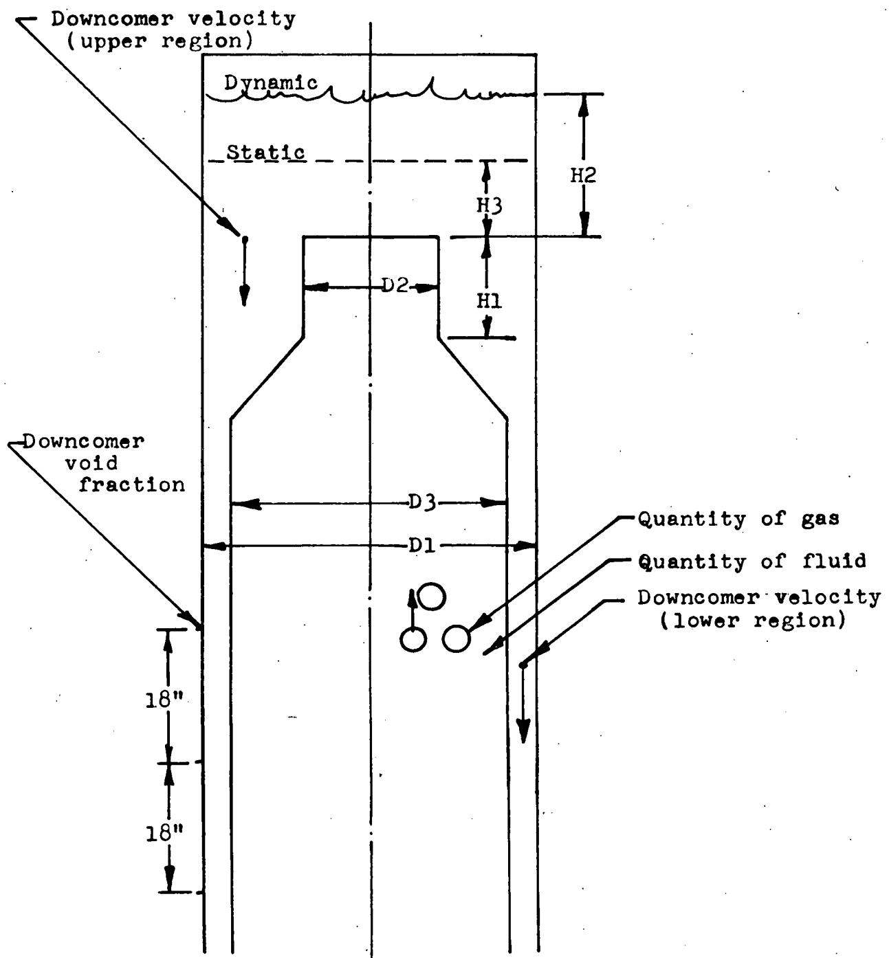
Figure 1 - Test Section Showing Parameters Under Investigation
