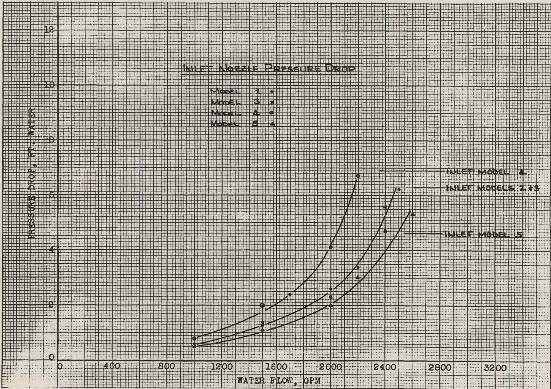
Figure 40 - Relative Performance of Inlet Nozzle
