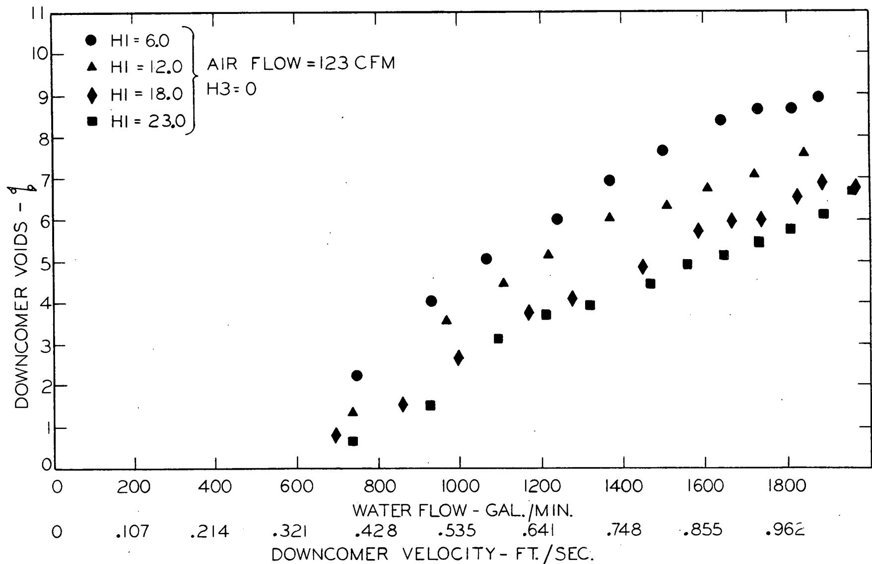
Figure 8 - Effect of Riser Length on Downcomer Voids (Loop Temp.  $150^{\circ}\text{F} \pm 10^{\circ}$ )
