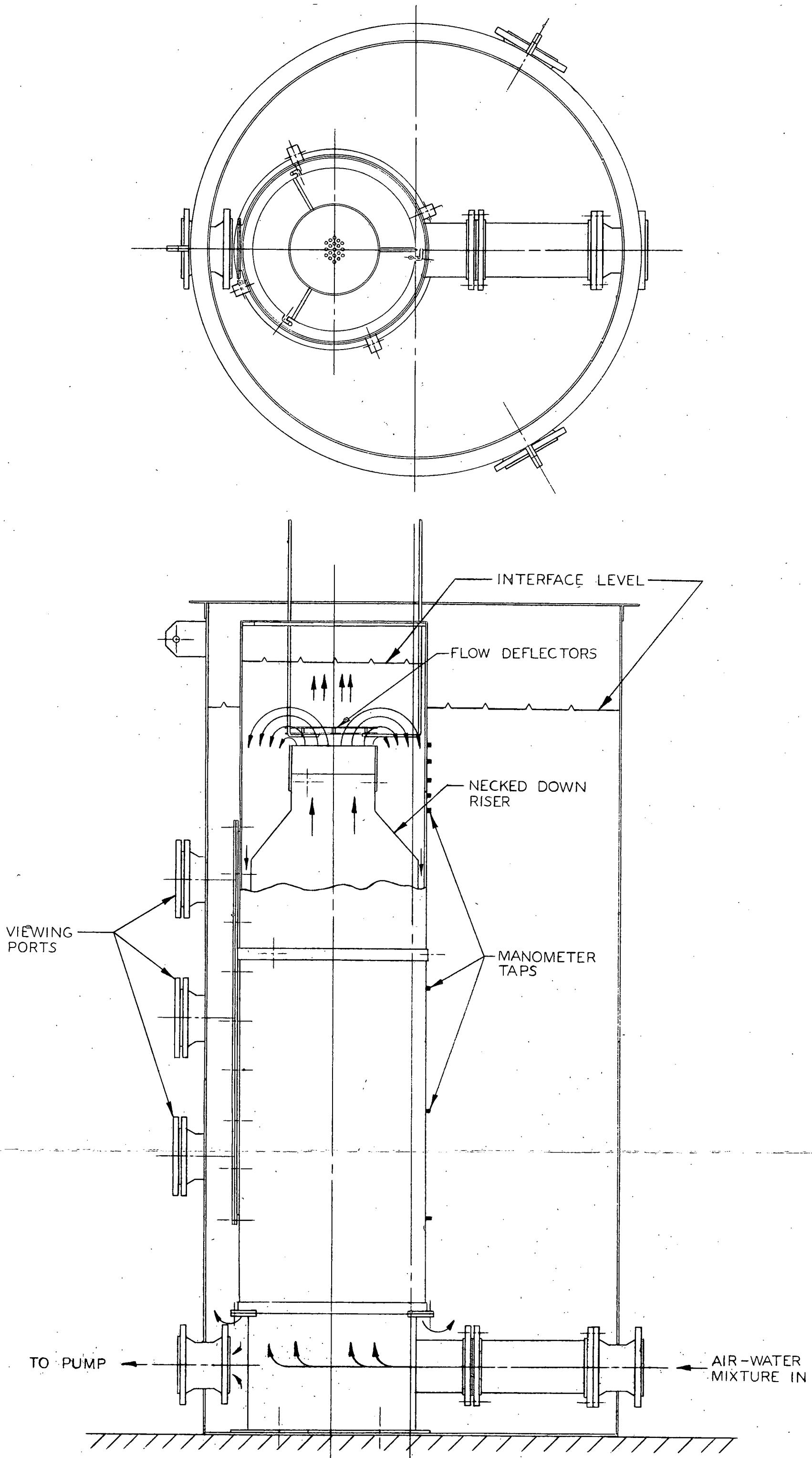
Figure I-A - Air-Water Tank Tests
