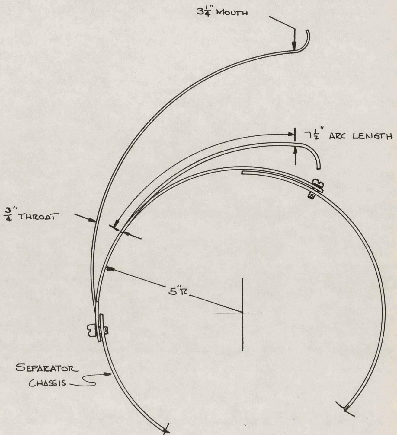
Figure 36 - Inlet Nozzle Model 4
