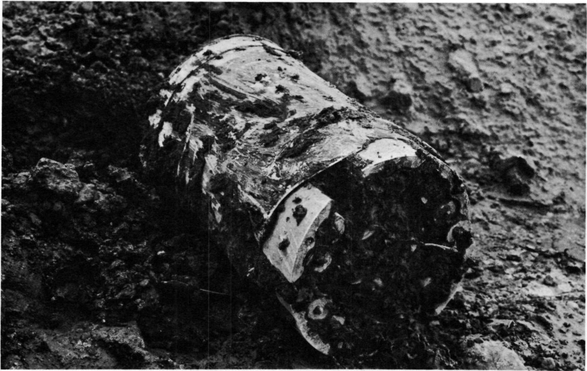
7611-5506 Figure 18. Reactor Vessel After Nose-On Water Impact Test
