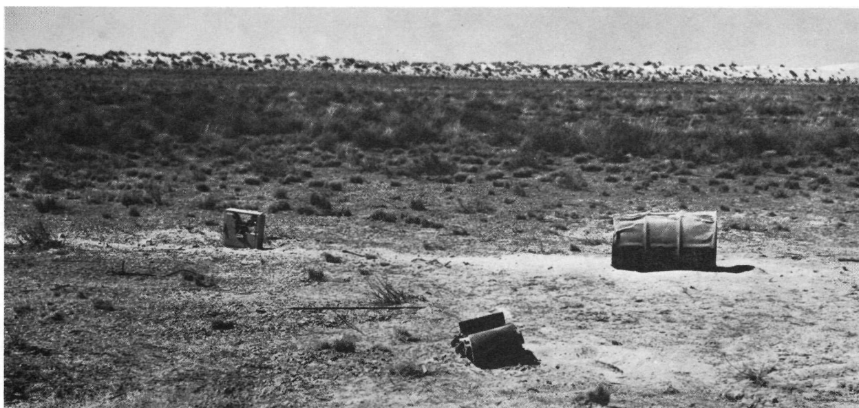
Figure 5. Pieces of Test Article After Explosion Test 7611-5517
