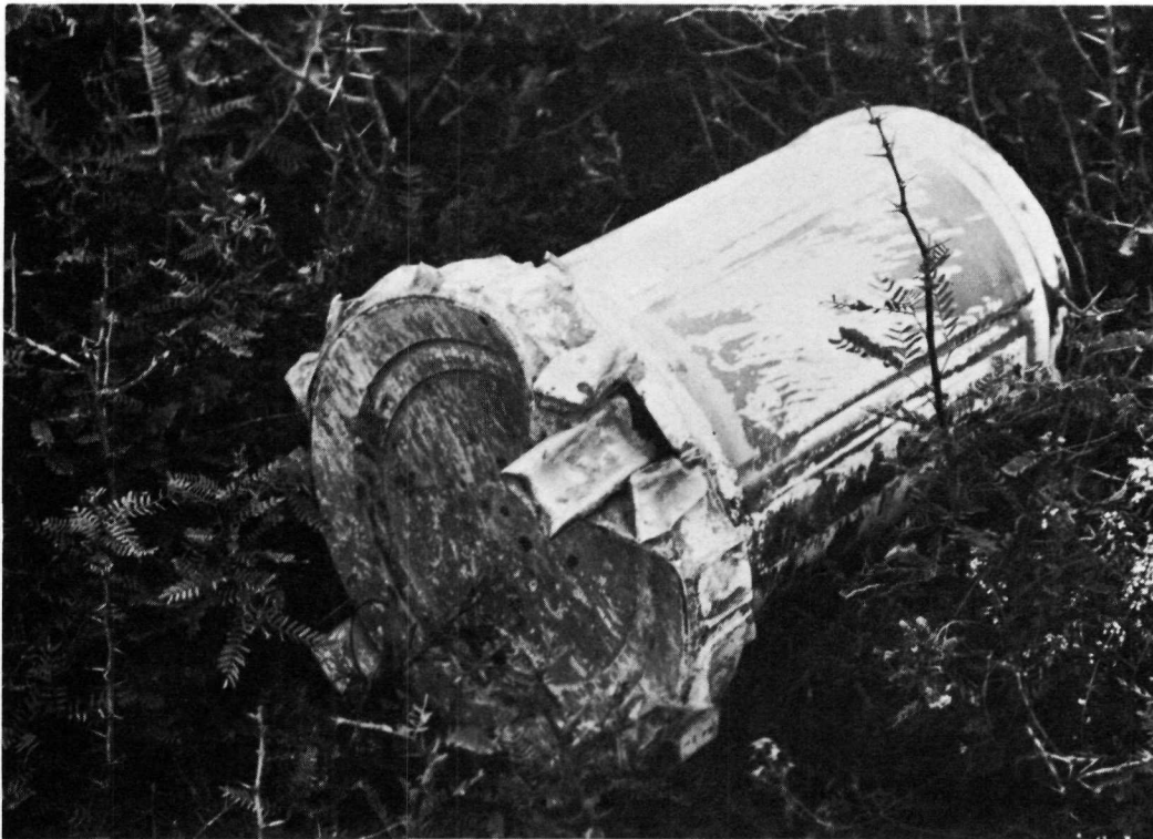
7611-5507 Figure 16. Reactor Vessel After Side-On Water Impact Test
