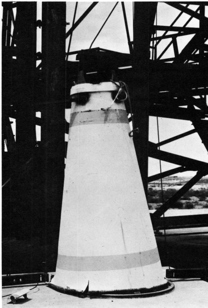
7611-5509 Figure 10. Test Article After 100-ft, Tail-On Drop Test
