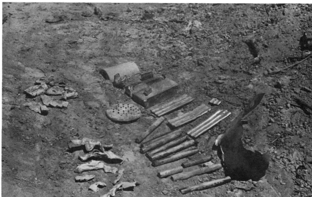
7568-0284 Figure 21. Pieces of Test Article Recovered After Concrete Impact Test
