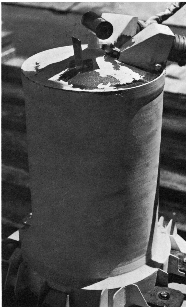
Figure 3. Test Article After LOX-NaK Interaction Test
