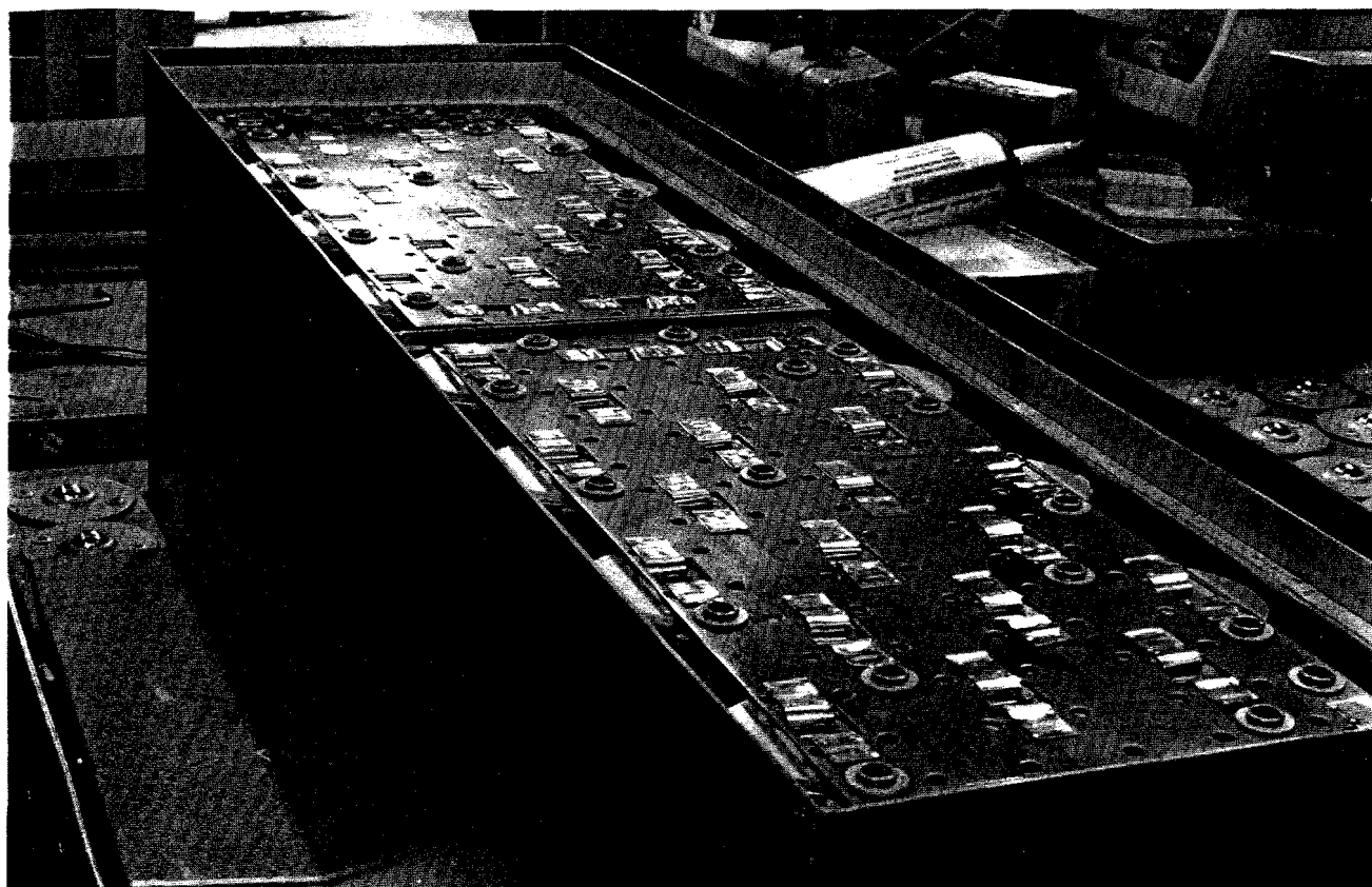
Figure 3-9 Two Bank ETX IIs Test Module
