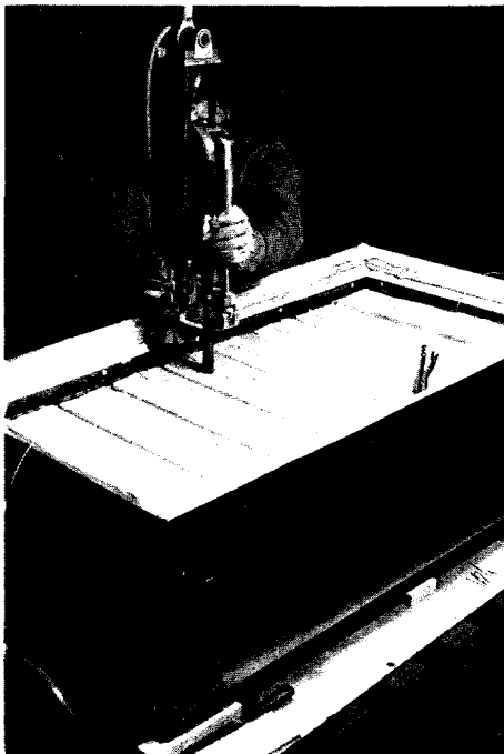
Welding of Bus-side Plates
