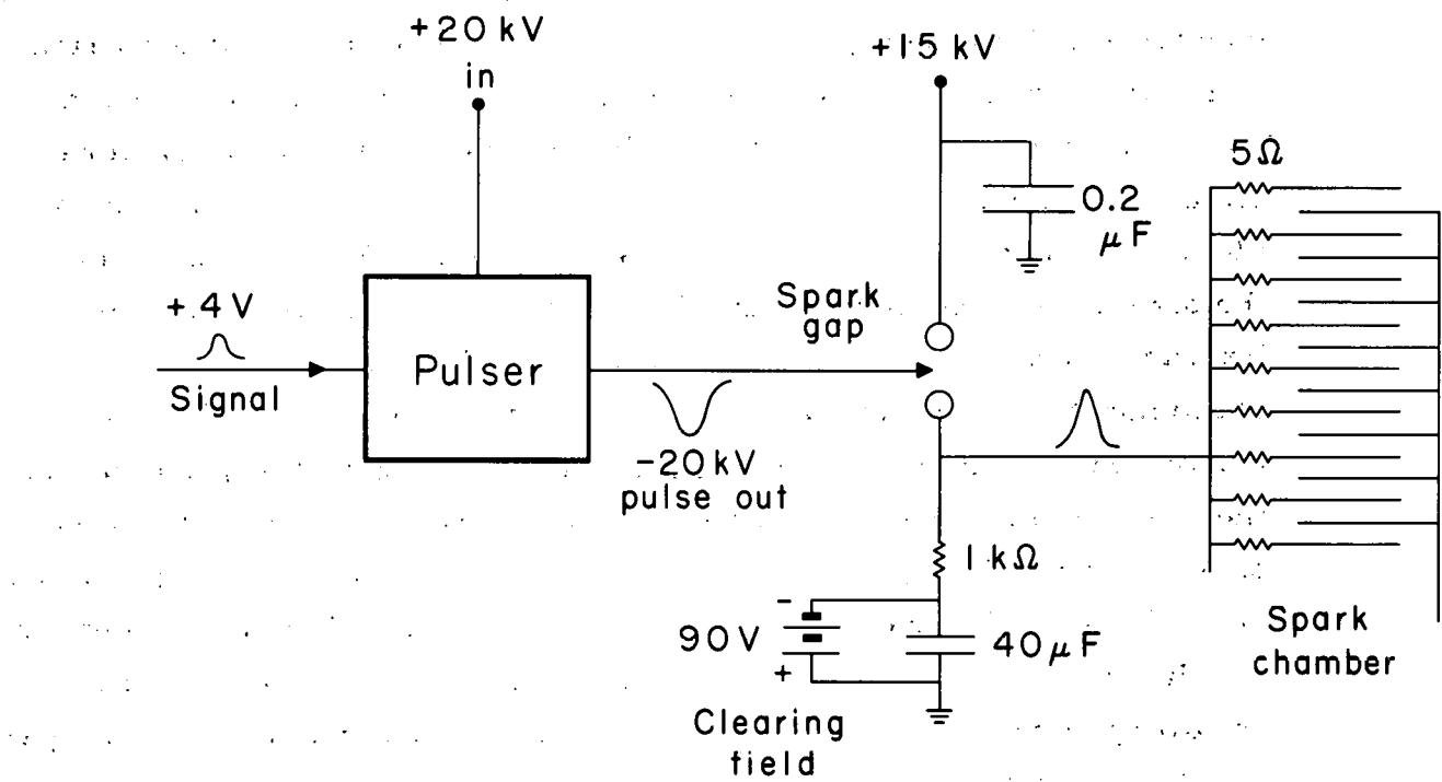
Fig. 7. System used to fire the spark chambers on a given signal from the counter electronics.
