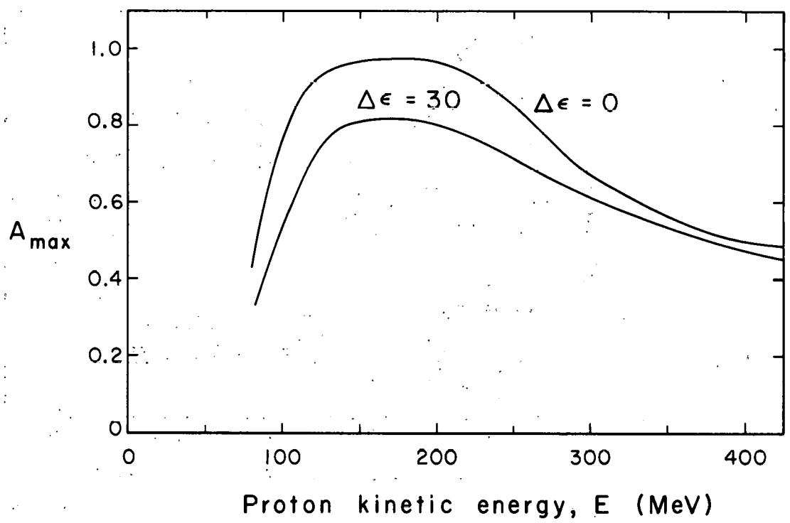
Fig. 13.  $A_{\max}$  as a function of incident-proton kinetic energy.  $A_{\max}$  is the largest magnitude the analyzability  $A$  ever attains between zero degrees and the diffraction minimum for incoming protons of a given energy.
