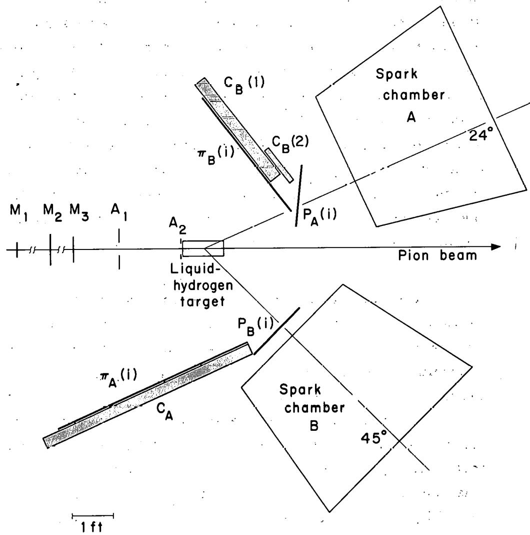
Fig. 3. Plan view of this experiment, showing the orientation of spark chambers and counters used to select desired events.
