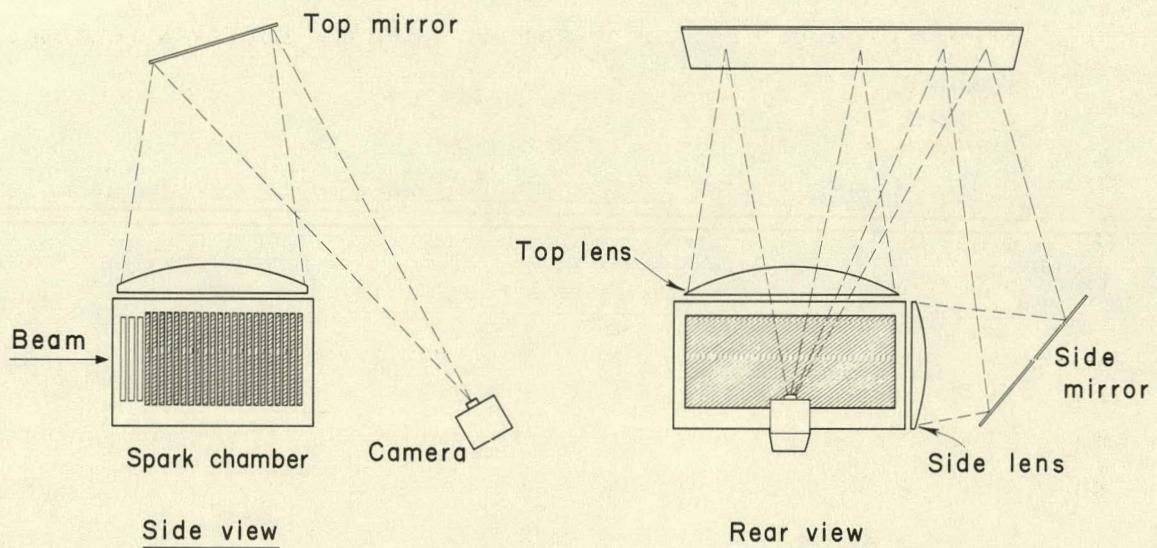
Fig. 9. Diagram of spark-chamber optics used to photograph the selected proton events.
