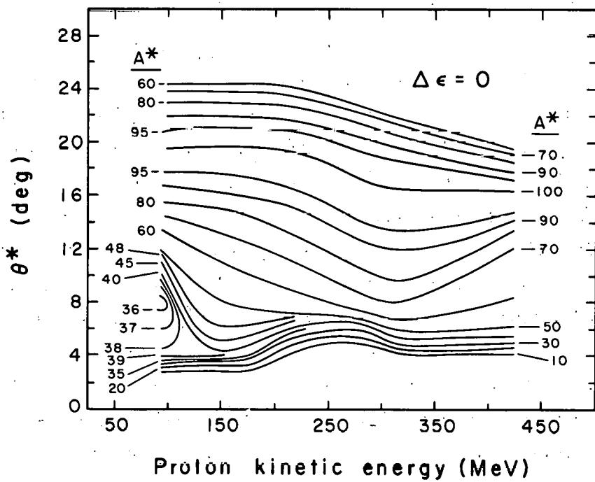
Fig. 11. Curves of constant  $A^*$  for elastic scattering ( $\Delta\epsilon = 0$ ) of protons from carbon as a function of laboratory-system energy and  $\theta^*$ , where  $\theta^*$  and  $A^*$  are related to laboratory scattering angle ( $\theta_{\text{lab}}$ ) and analyzability  $A$  by
