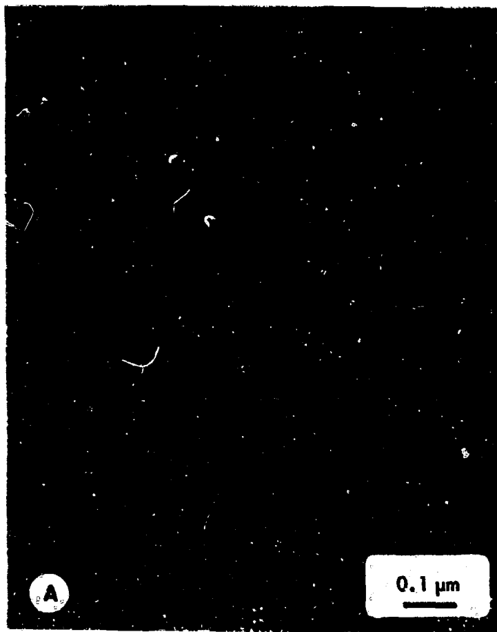
Fig. 3. Examples of the Two Components of Microstructural Damage Seen in BBC Metals Irradiated in the Temperature Range 0.3 to 0.5 T_m . This is a sample of molybdenum irradiated at 585°C to 2.5 \times 10^{22} \text{ n/cm}^2 ( E > 0.1 \text{ MeV} ). (a) Shows voids seen under absorption contrast conditions. (b) Dislocation loops and segments seen under diffraction contrast conditions. Both components of damage occur throughout the specimen.
