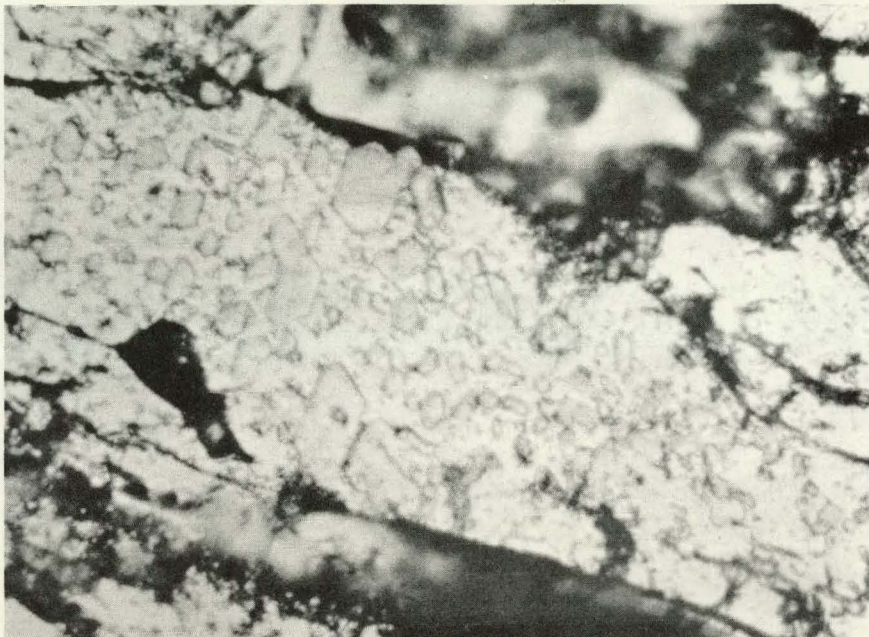
Figure 64. SPECIMEN V-2-P, POLYGON SHAPED CRYSTALS WITHIN COLUMNAR STRUCTURE
