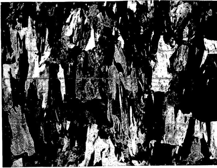
Figure 2. Grain Structure of Alpha Plutonium Polarized Illumination X250
