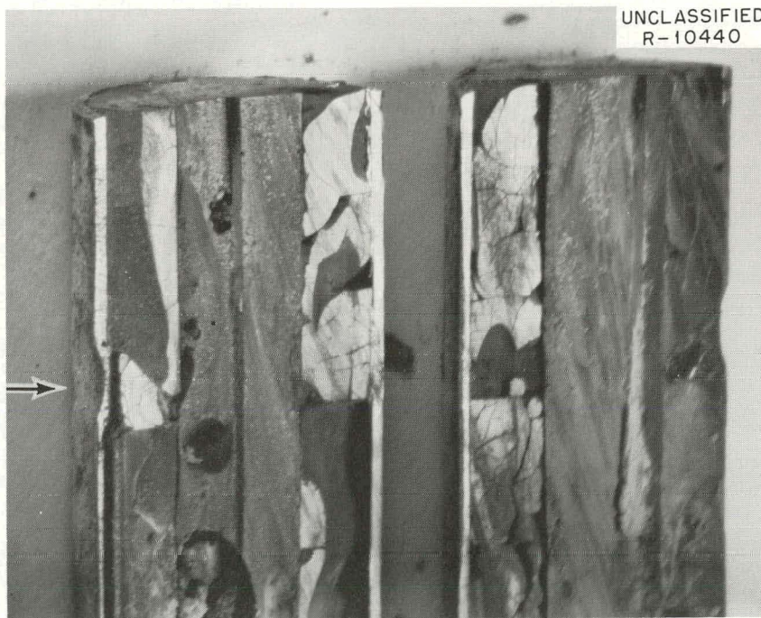
Fig. 4.2. Cracked \text{UO}_2 Pellets from Capsule 07-5. The depression and fracture pattern at the pellet-to-pellet interface is indicated by the arrow. Mating halves of the capsule are shown.
