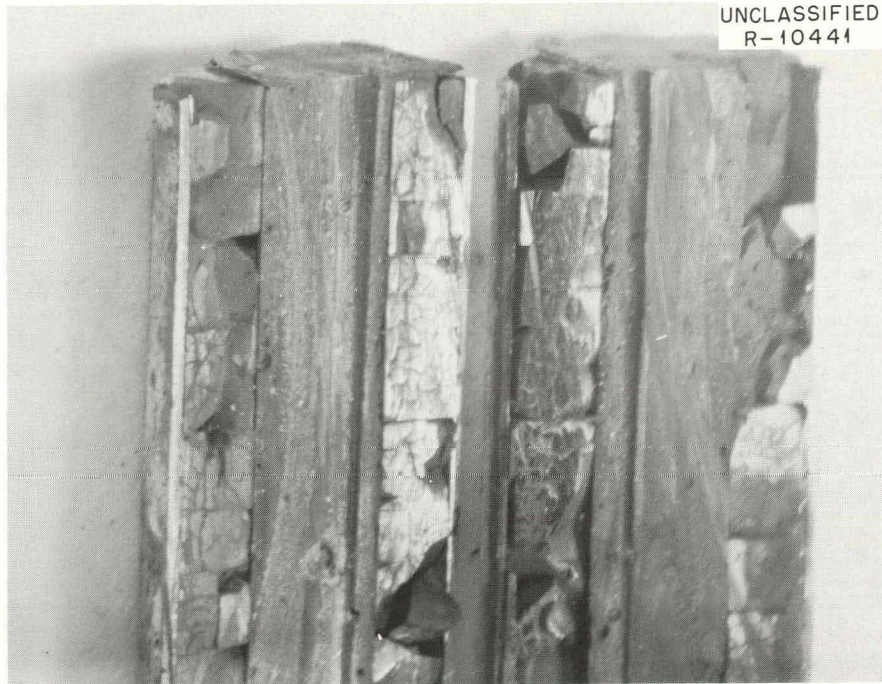
Fig. 4.1. Cracked \text{UO}_2 Pellets in Capsule 02-5. The central void was filled with epoxy resin. Mating halves of the capsule are shown.
