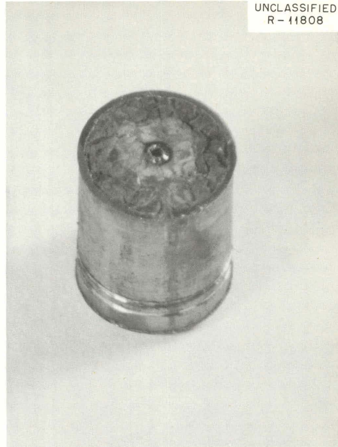
Fig. 7.3. Transverse Section of Capsule 06-5. Note sintered fuel surrounding central thermocouple.
