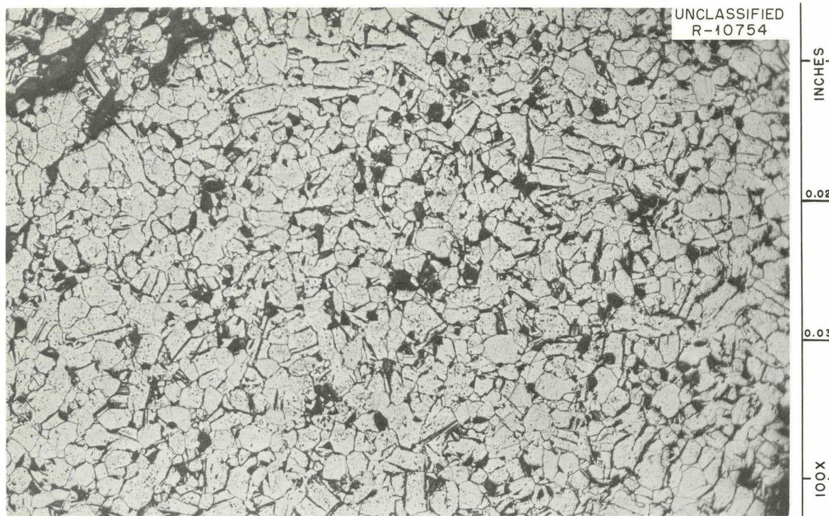
Fig. 8.12. Irradiated Cold-Pressed and Sintered BeO Specimen 7-l-5, Which Was Exposed to a Fast-Neutron ( >1 Mev) Dose of 1.20 \times 10^{21} Neutrons/cm 2 at 583°C in Experiment 41-7. As polished.
