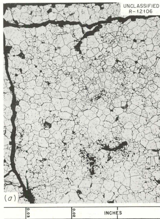
Fig. 4.20. Microstructure of a \text{UO}_2 Pellet from Capsule E-4. Etched. 100X. (a) Outer surface region. (b) Mid-radius region. (c) Edge of central void that formed during irradiation.
