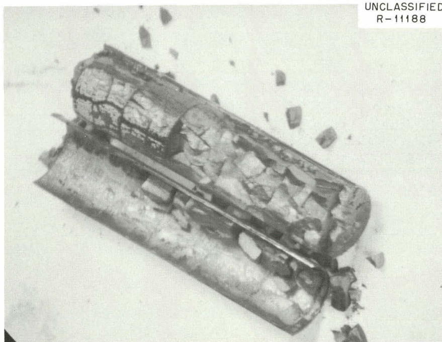
Fig. 4.7. UO 2 Pellets from Capsule 04-5 Showing White "NaK" Deposit.
