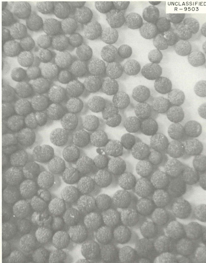
Fig. 6.8. Pyrolytic-Carbon-Coated Uranium Carbide Particles with Columnar-Type Coatings After Irradiation in Capsule B9-7 to a Burnup of 12 at. % Uranium at 1500 to 1650°F. 30X.
