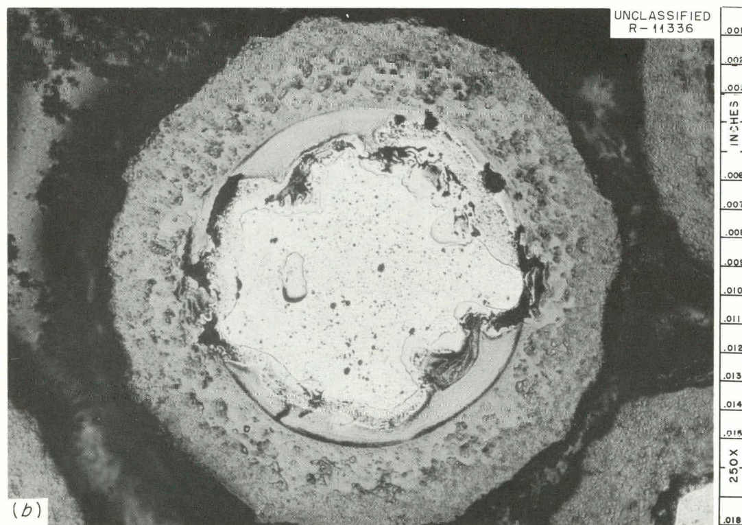
Fig. 6.11. Sectioned, Duplex-Type, Pyrolytic-Carbon-Coated Uranium Carbide Particles. (a) Unirradiated. (b) Irradiated at 30 at. % uranium burnup at 600 to 1750°F.
