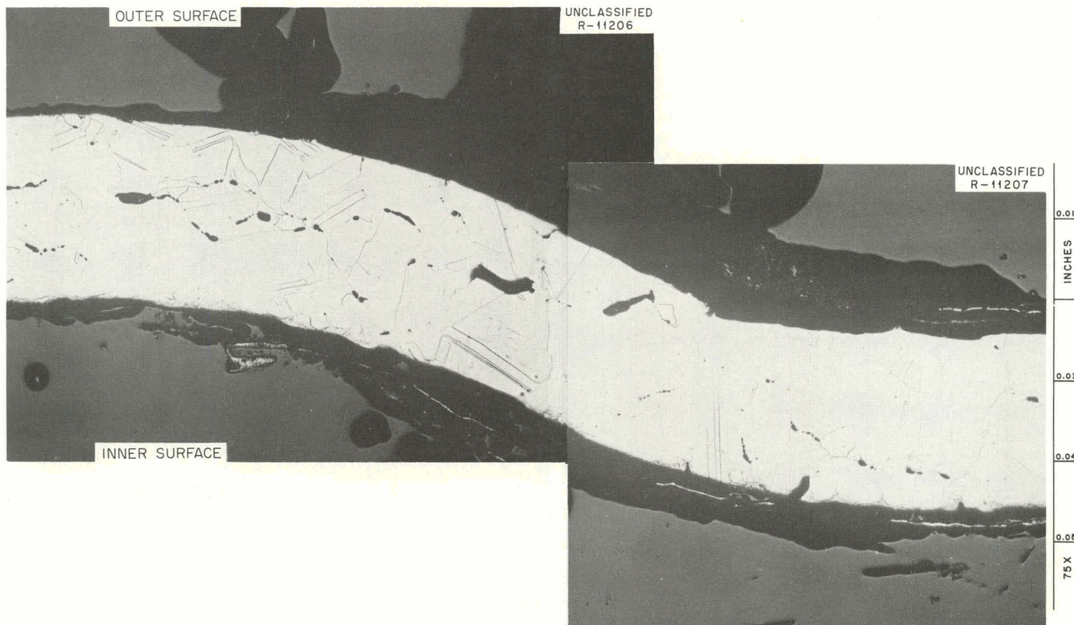
Fig. 4.5. Portion of Longitudinal Section Through the Depression in the Cladding of Capsule 07-5. Etched.
