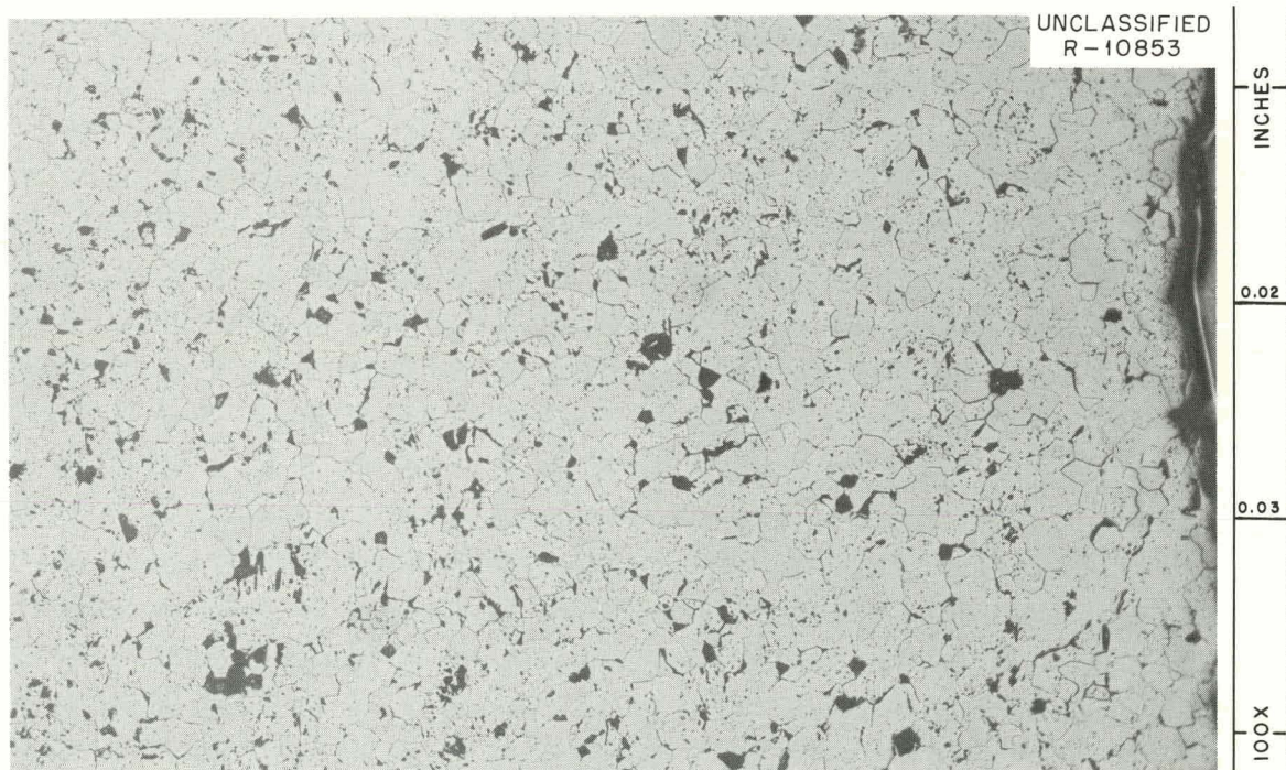
Fig. 8.11. Irradiated Cold-Pressed and Sintered BeO Specimen 7-8-2, Which Was Exposed to a Fast-Neutron ( >1 Mev) Dose of 2.25 \times 10^{21} Neutrons/cm 2 at 1100°C in Experiment 41-7. As polished.
