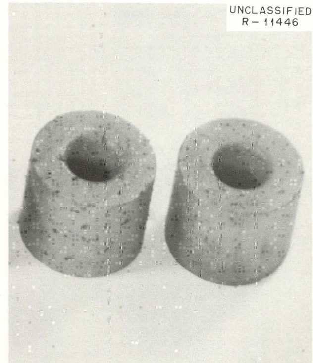
Fig. 6.4. Typical Fuel Pellets from Capsule 08A-5 After Removal of Graphite Sleeve. 2X.
