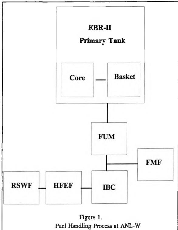
storage and subsequent processing in the FCF is a multi-stage process, involving complex operations at a minimum of four different facilities at the ANL-W site. The process is shown schematically in Figure 1.
