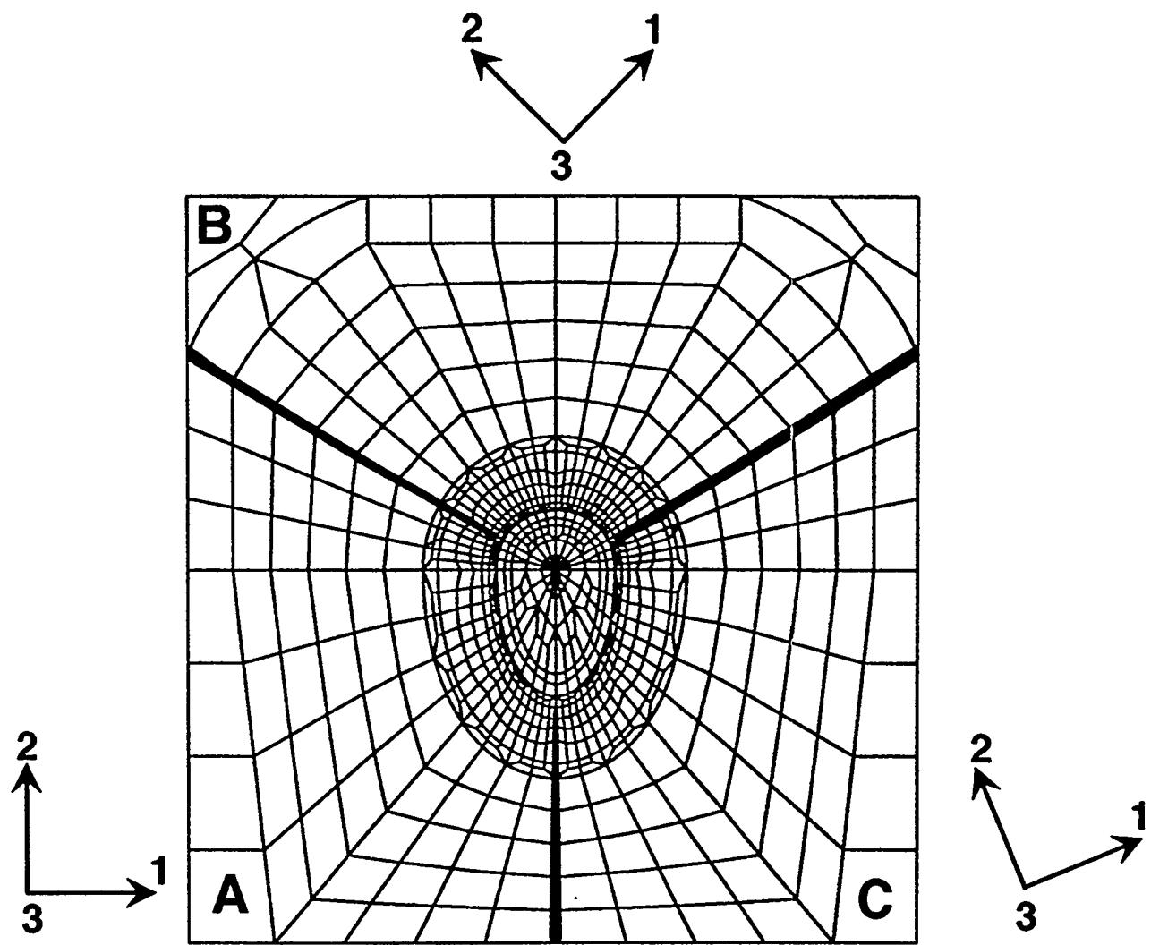
FIGURE 1. MODEL OF CARBIDE PRECIPITATE AT GRAIN BOUNDARY TRIPLE POINT
