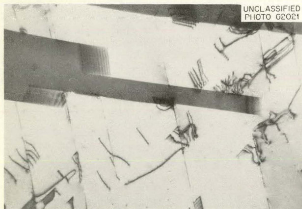
Fig. 15.21. Electron Transmission Photomicrograph of a Cu-15 at. % Al Foil Irradiated at 100^\circ\text{C} to 10^{16} Neutrons/ \text{cm}^2 ( >0.6 Mev). The dislocation structures to be noted here are believed to have been introduced primarily during preparation of the foil.
