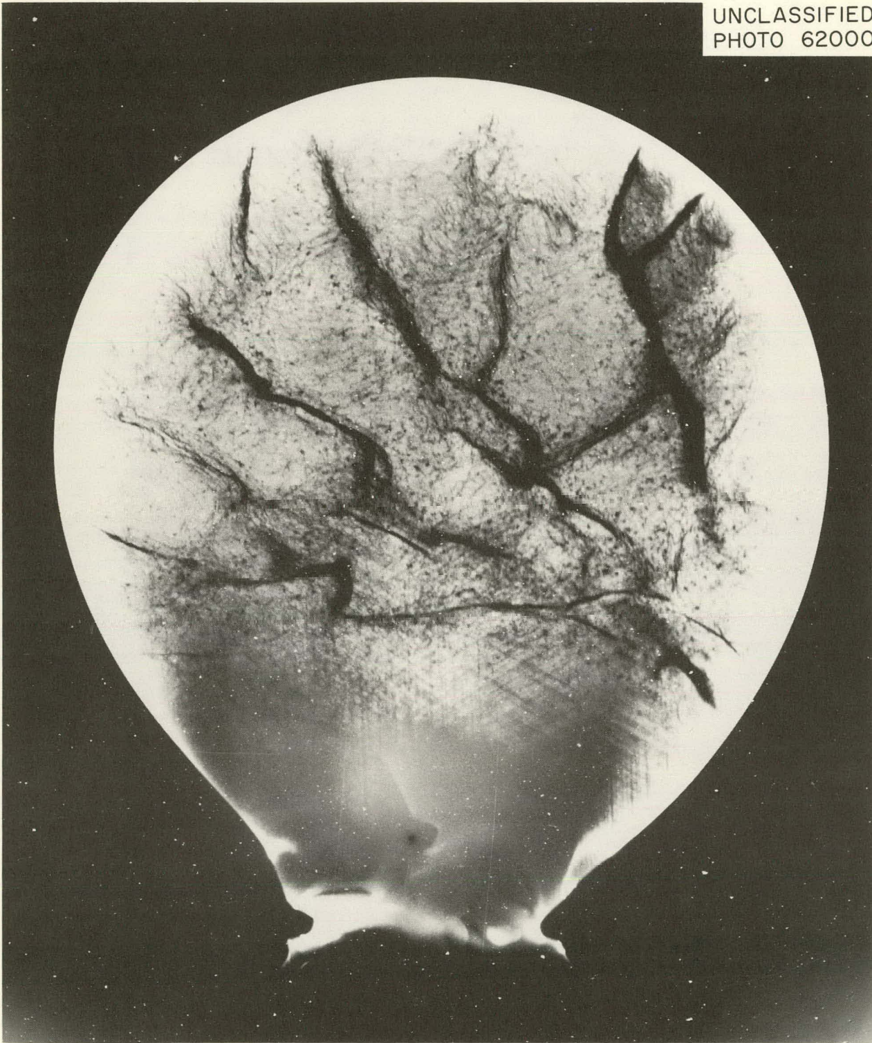
Fig. 8.1. X-Ray Topograph of a Copper Crystal Obtained with Anomalous Transmission. 5X. Reduced 16%.
