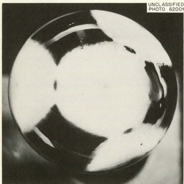
Fig. 8.5. Single-Crystal Sphere of Copper After Four Weeks in 0.2 \text{ M CuSO}_4 . Light areas in the photograph represent faceted crystal areas. Note the large un-faceted area around (100) poles.
