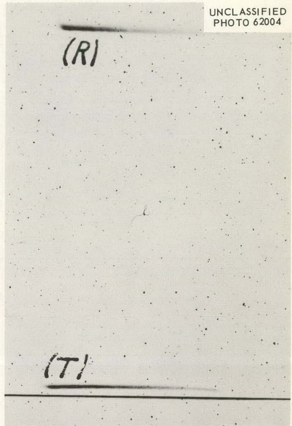
Fig. 4.2. A 16-hr Exposure to Both Beams from Same Crystal as in Fig. 4.1. Upper line, anomalous reflected beam ( R ); middle line, anomalous transmitted beam ( T ); and lower line, direct beam with crystal removed. Ilford L-4 nuclear plate, 100- \mu emulsion; \lambda = 1.54 A. 3X.
