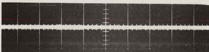
Figure 7.33 - Deflection with Single Phase Flow 190 GPM and 6.3 FPS e_x = 0.15 \text{ cm} \delta = 0.000054 \text{ in.}
