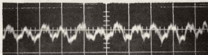
Figure 7.29 - Interference Frequency with 190 GPM Water Flow 5 cm = 0.1 sec f_i = 60 cps
